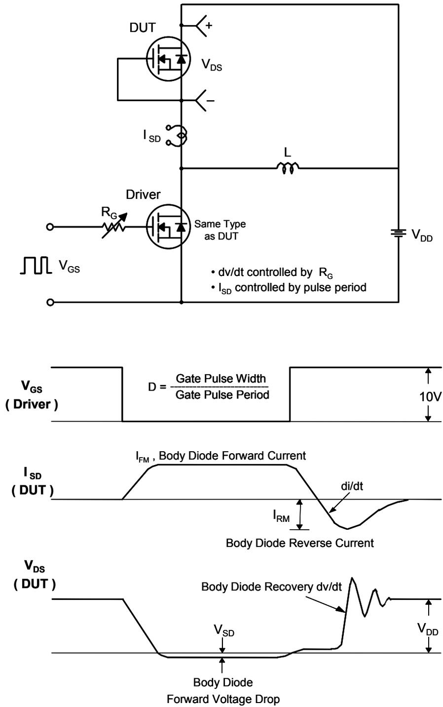
Figure 18. Peak Diode Recovery  $dv/dt$  Test Circuit & Waveforms
