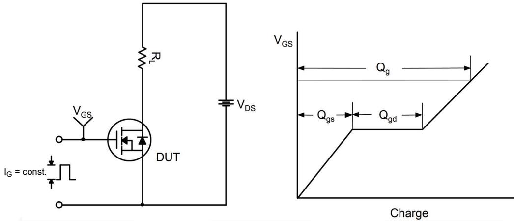
Figure 15. Gate Charge Test Circuit & Waveform
