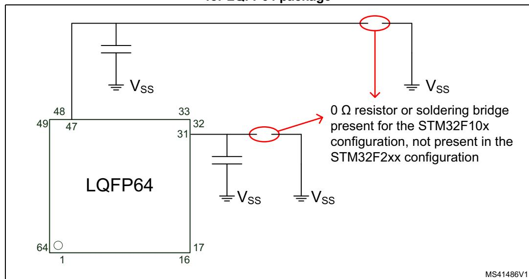
**Figure 2. Compatible board design between STM32F10x and STM32F2xx
