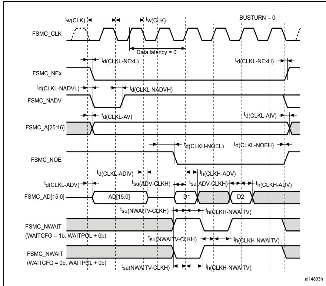
Table 75. Synchronous multiplexed NOR/PSRAM read timings<sup>(1)(2)</sup>
