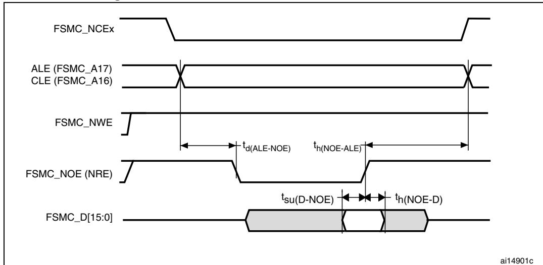
**Figure 70. NAND controller waveforms for write access**
