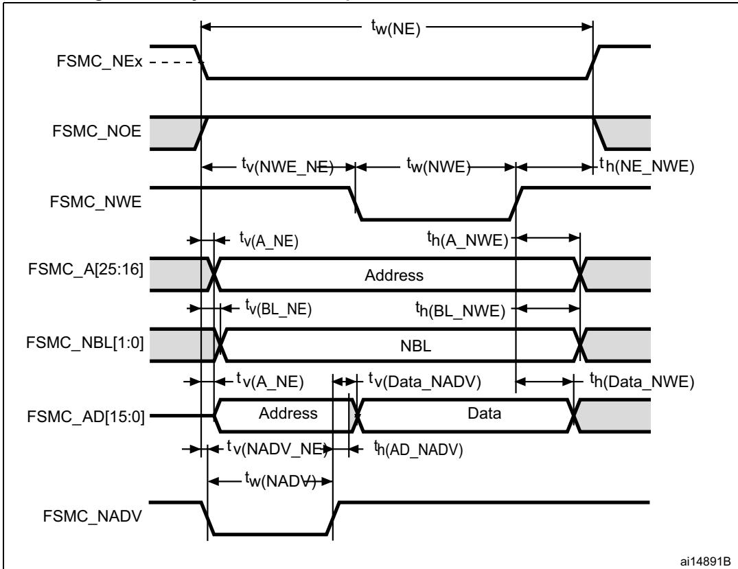
**Table 74. Asynchronous multiplexed PSRAM/NOR write timings<sup>(1)(2)</sup>**
