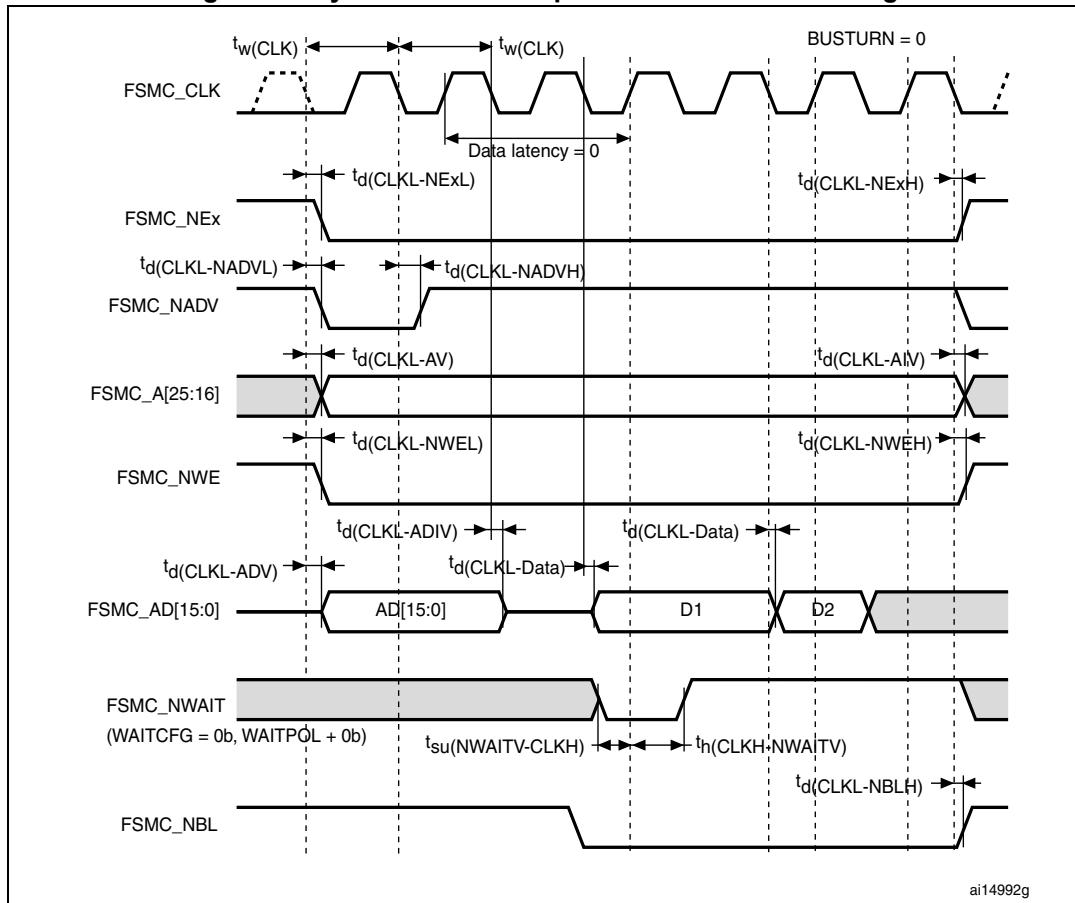
**Table 76. Synchronous multiplexed PSRAM write timings<sup>(1)(2)</sup>**
