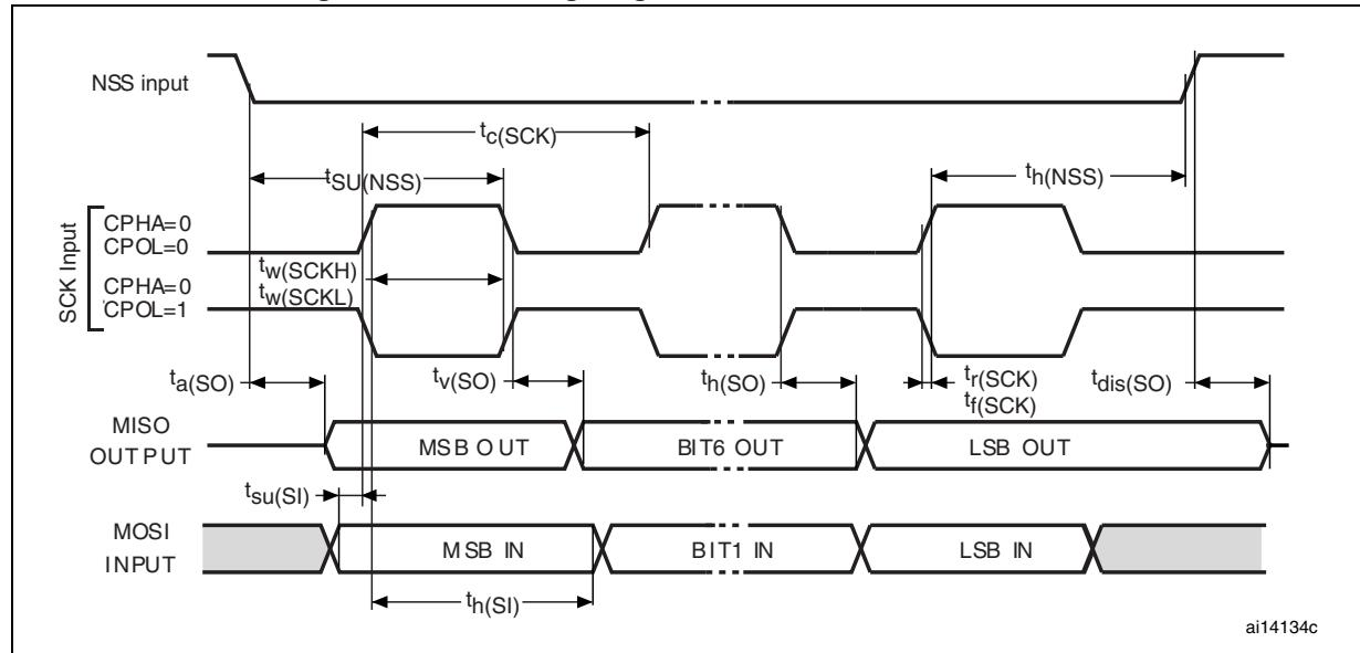
Figure 41. SPI timing diagram - slave mode and CPHA = 1
