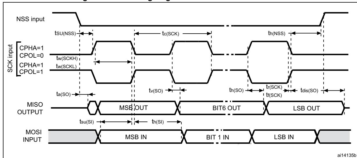
Figure 42. SPI timing diagram - master mode
