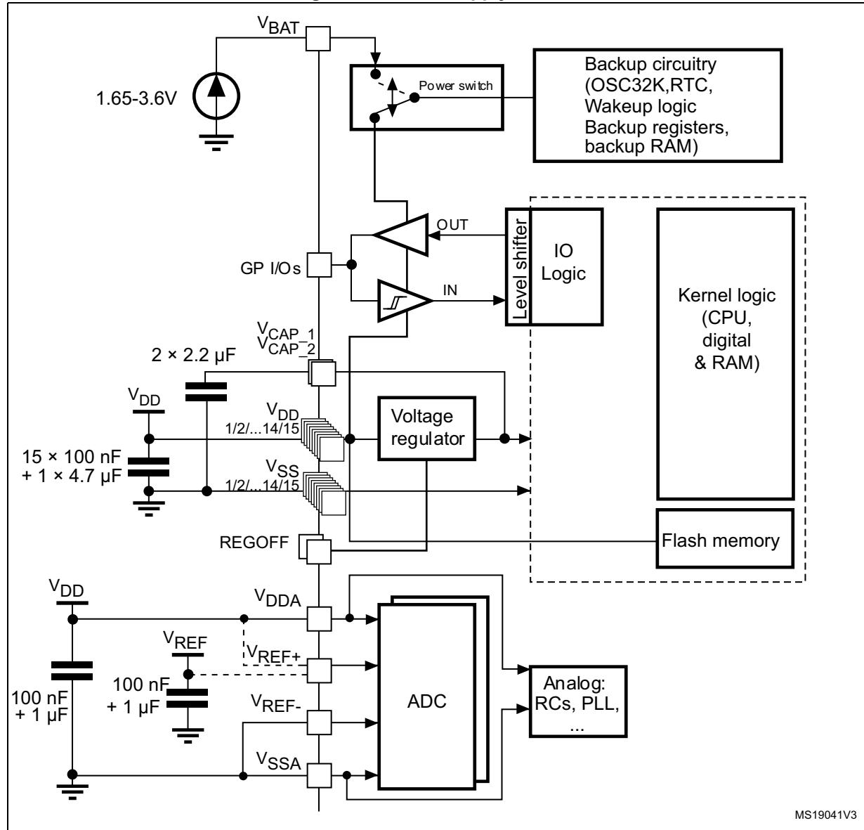
1. Each power supply pair must be decoupled with filtering ceramic capacitors as shown above. These capacitors must be placed as close as possible to, or below, the appropriate pins on the underside of the PCB to ensure the good functionality of the device.
