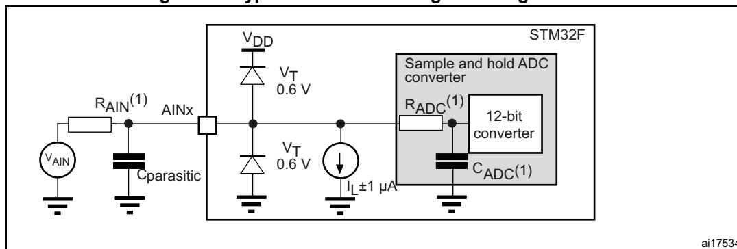
1. Refer to [Table 65](#) for the values of  $R_{AIN}$ ,  $R_{ADC}$  and  $C_{ADC}$ .
