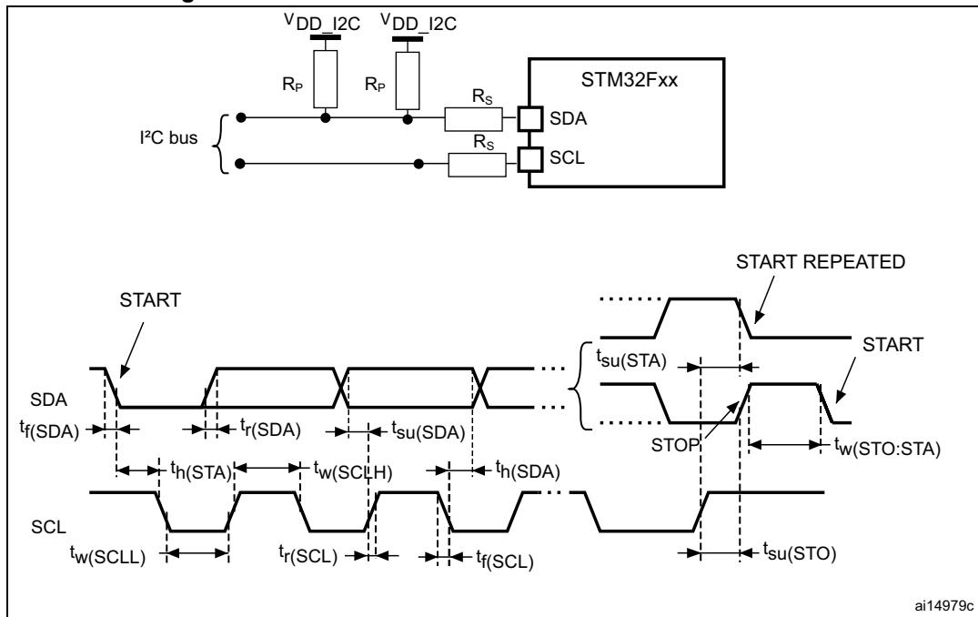
1.  $R_S$  = series protection resistor.
