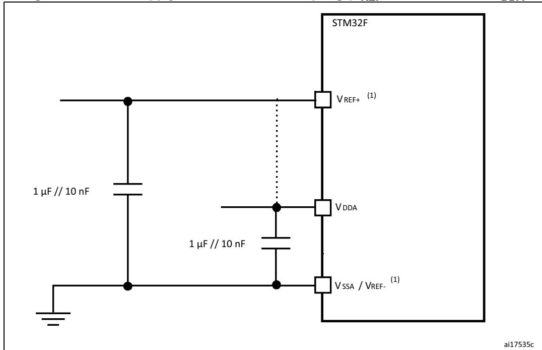
1.  $V_{REF+}$  and  $V_{REF-}$  inputs are both available on UFBGA176 package.  $V_{REF+}$  is also available on all packages except for LQFP64. When  $V_{REF+}$  and  $V_{REF-}$  are not available, they are internally connected to  $V_{DDA}$  and  $V_{SSA}$ .
