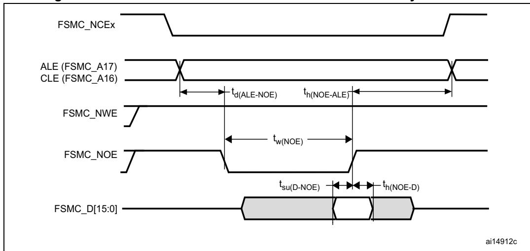
**Figure 72. NAND controller waveforms for common memory write access**
