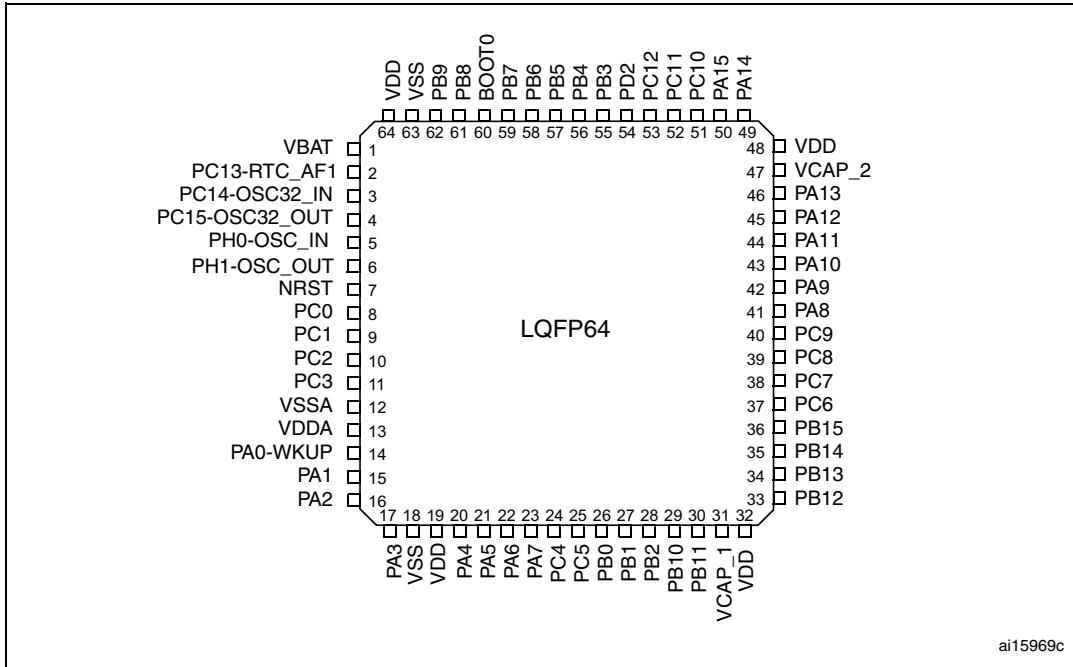
1. The above figure shows the package top view.
