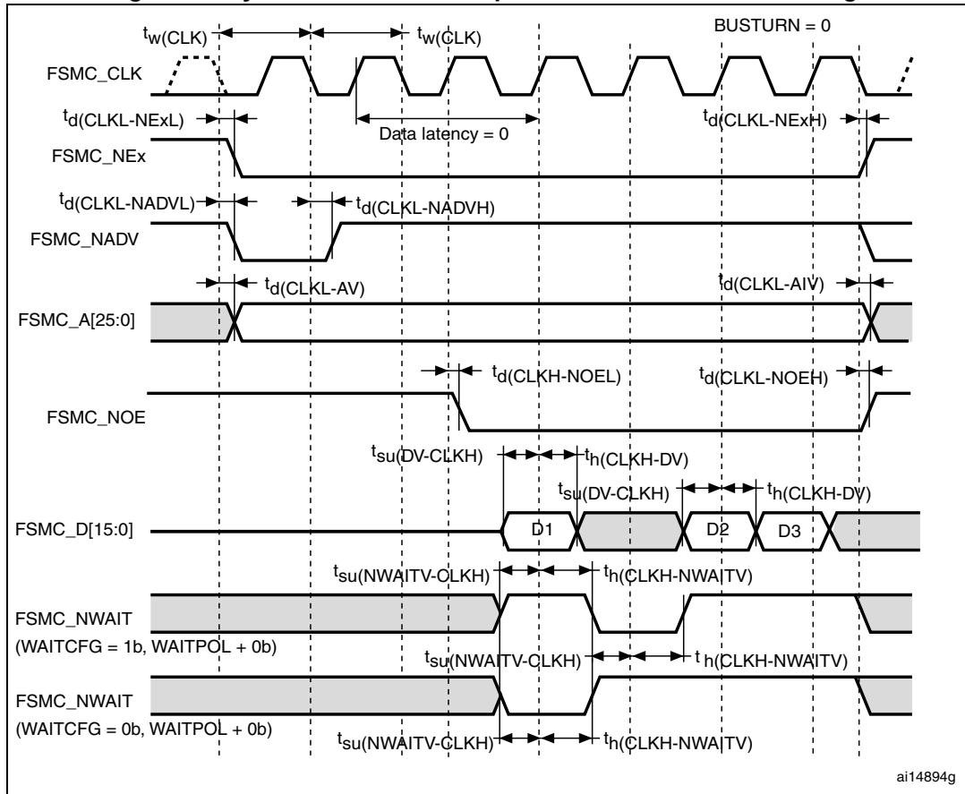
**Table 77. Synchronous non-multiplexed NOR/PSRAM read timings<sup>(1)(2)</sup>**
