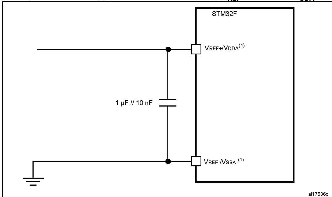
1.  $V_{REF+}$  and  $V_{REF-}$  inputs are both available on UFBGA176 package.  $V_{REF+}$  is also available on all packages except for LQFP64. When  $V_{REF+}$  and  $V_{REF-}$  are not available, they are internally connected to  $V_{DDA}$  and  $V_{SSA}$ .
