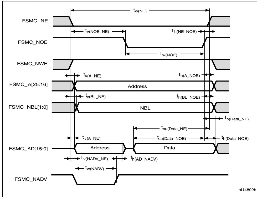
Table 73. Asynchronous multiplexed PSRAM/NOR read timings<sup>(1)(2)</sup>
