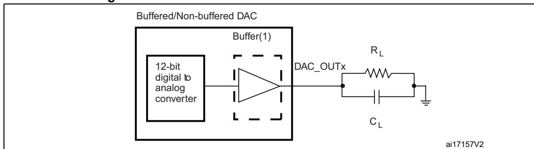
1. The DAC integrates an output buffer that can be used to reduce the output impedance and to drive external loads directly, without the use of an external operational amplifier. The buffer can be bypassed by configuring the BOFFx bit in the DAC\_CR register.
