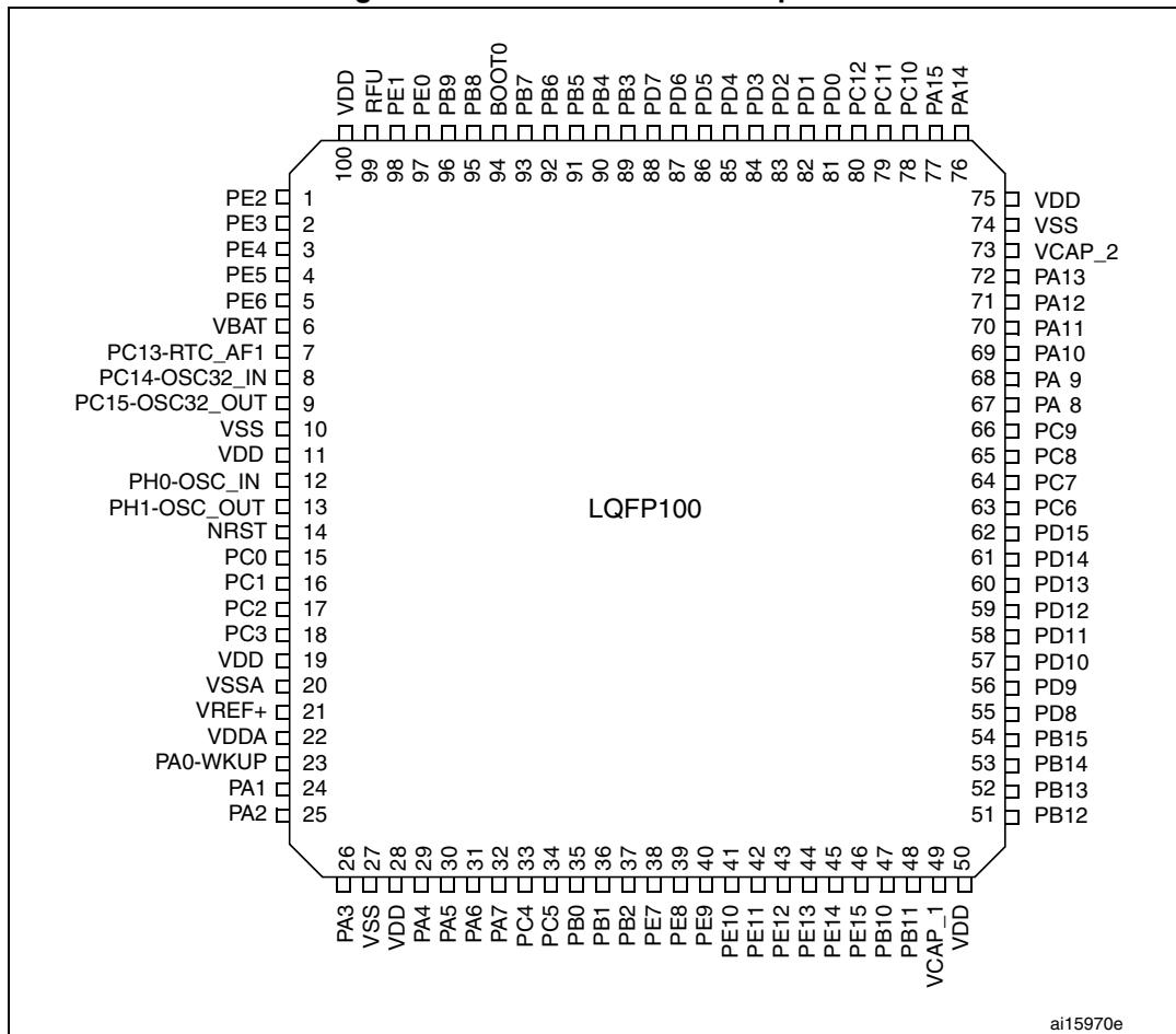
1. RFU means "reserved for future use". This pin can be tied to V<sub>DD</sub>, V<sub>SS</sub> or left unconnected.
