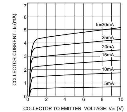
Fig.10 Output characteristics
