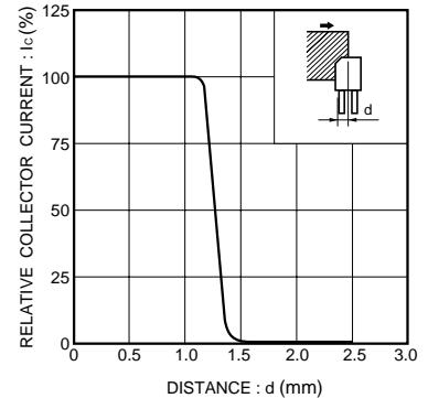
Fig.1 Relative output current vs. distance (I)
