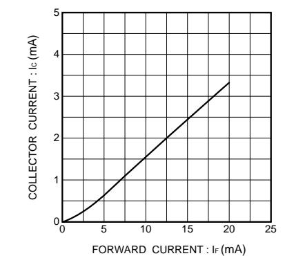
Fig.7 Collector current vs. forward current
