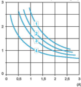
AC- Control of weak electromagnetic loads of electromagnets  $\leq 72$  VA (make:  $\cos \phi = 0.3$ , break:  $\cos \phi = 0.3$ )
