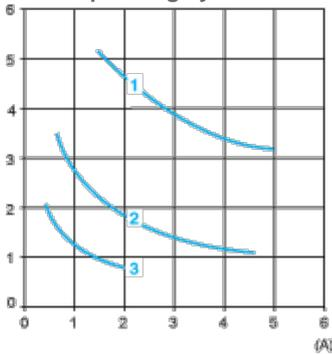
DC- Control of resistive loads and isolated solid state loads via optocoupler ( $L/R \leq 1$  ms)
