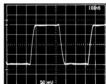
Figure 22c. Unity Gain Inverter Small Signal Pulse Response
