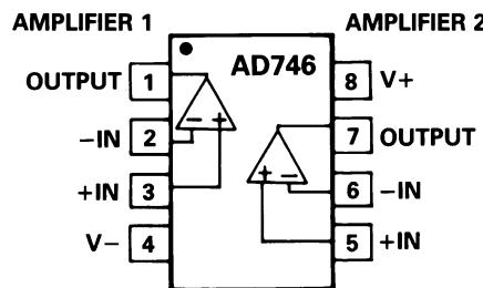
The AD746 is available in three 8-pin packages: plastic mini DIP, hermetic cerdip and surface mount (SOIC).
