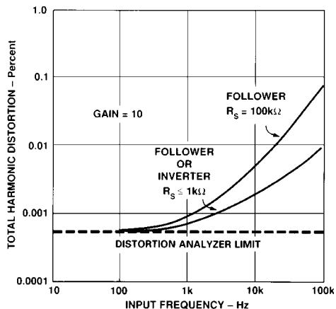
Figure 28. THD vs. Frequency Using Standard Distortion Analyzer
