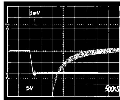
Figure 25. Settling Time of the 3 Op Amp Instrumentation Amplifier.
