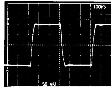
Figure 21c. Gain of 2 Follower Small Signal Pulse Response
