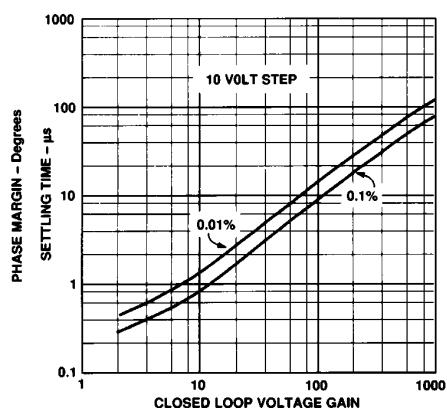
Figure 11. Settling Time vs. Closed Loop Voltage Gain
