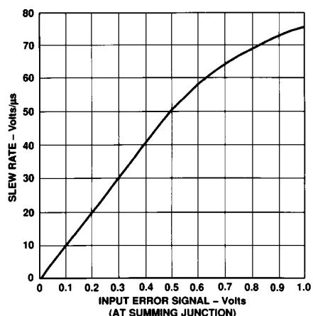
Figure 18. Slew Rate vs. Input Error Signal
