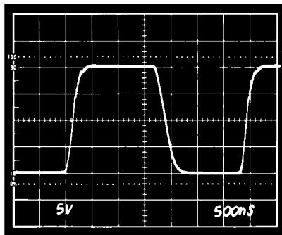
Figure 24. Pulse Response of the 3 Op Amp Instrumentation Amplifier.
