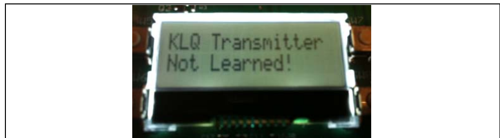
FIGURE 2-3: ERROR MESSAGE OF RECEIVING PACKET FROM UNKNOWN TRANSMITTER
