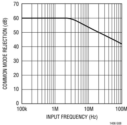
**Figure 7. Common Mode Rejection vs Input Frequency**
