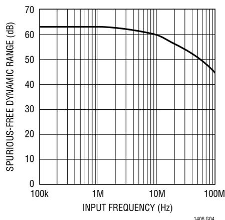
Figure 6. Spurious-Free Dynamic Range vs Input Frequency
