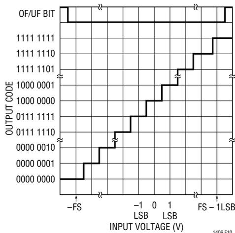
Figure 10. Transfer Characteristics
