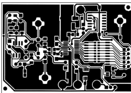
Figure 12c. Suggested Evaluation Circuit Board—Component Side Layout
