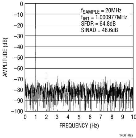
Figure 2a. Nonaveraged, 4096 Point FFT Input Frequency = 1MHz
