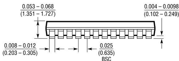
\* DIMENSION DOES NOT INCLUDE MOLD FLASH. MOLD FLASH SHALL NOT EXCEED 0.006" (0.152mm) PER SIDE
