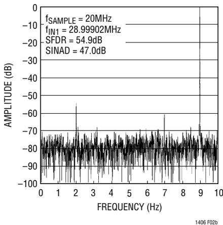
Figure 2b. Nonaveraged, 4096 Point FFT Input Frequency = 30MHz
