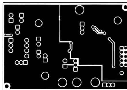
Figure 12d. Suggested Evaluation Circuit Board—Solder Side Layout
