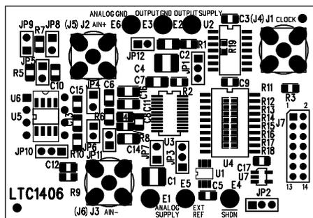
Figure 12b. Suggested Evaluation Circuit Board—Component Side Silkscreen
