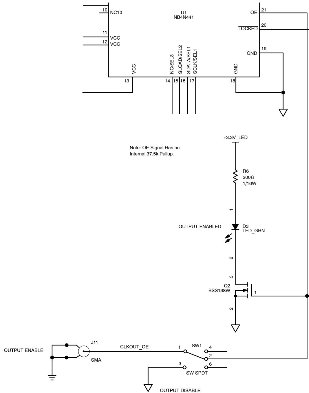
Figure 6. Output Enable
