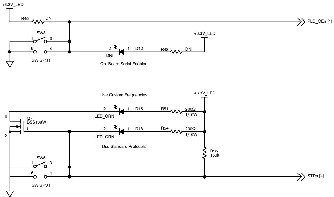
Figure 10. Output Enable
