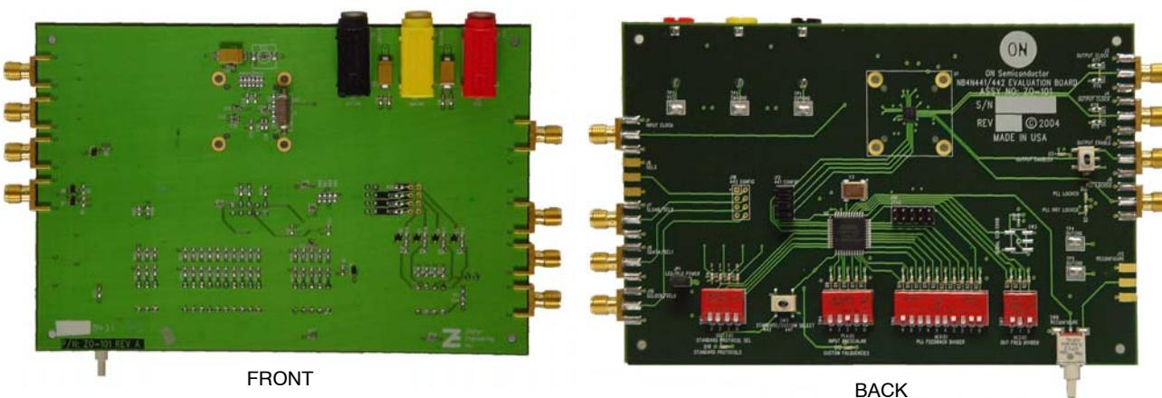
Figure 1. NB4N441MNGEVB Evaluation Board
