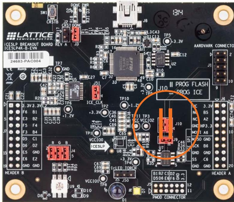
3. Connect the iCE40 Ultra breakout board via the USB cable to a PC or MAC.
