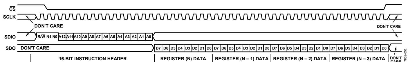
Figure 65. Serial Control Port Read—MSB First, 16-Bit Instruction, Four Bytes of Data
