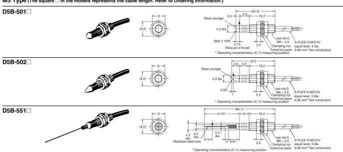
Note: 1. Unless otherwise specified, a tolerance of ±0.4 mm applies to all dimensions.
