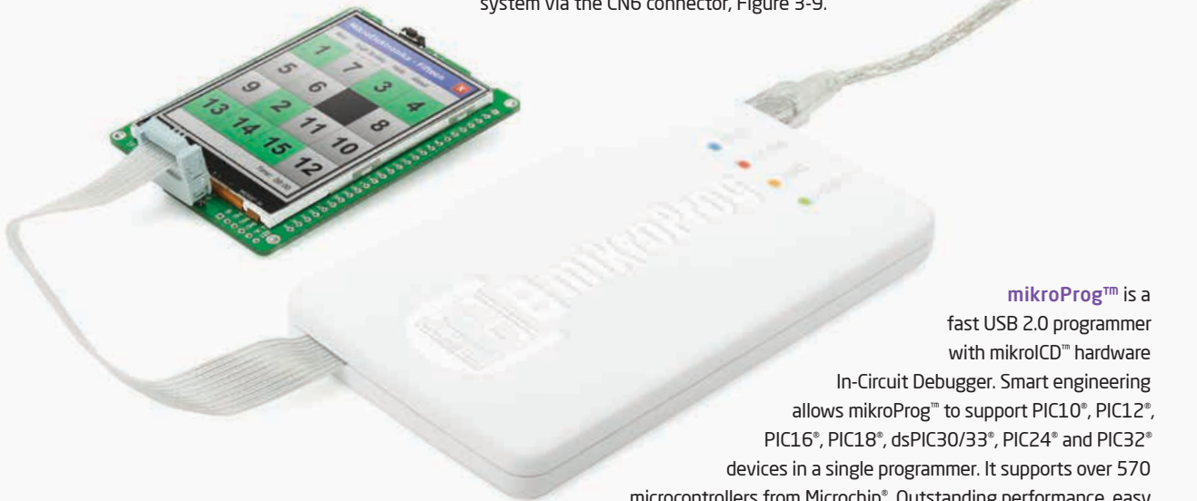
Figure 3-9: Connecting mikroProg™ to mikroMedia™
