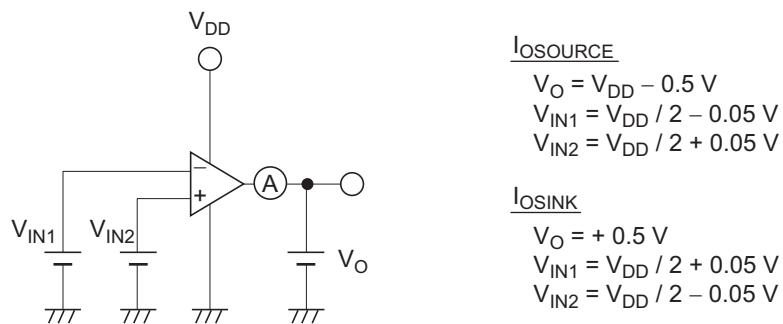
7. Common Mode Input Voltage,  $V_{CM}$  & Common Mode Rejection Ratio, CMRR
