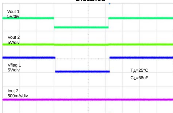
Channel 1 Enabled and Shorted with Channel 2 Disabled
