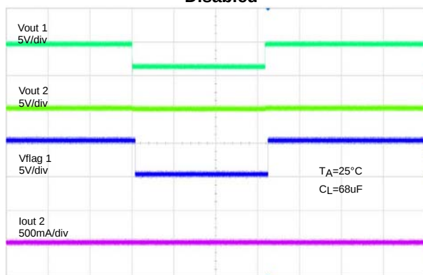
Channel 1 Enabled and Shorted with Channel 2 Disabled
