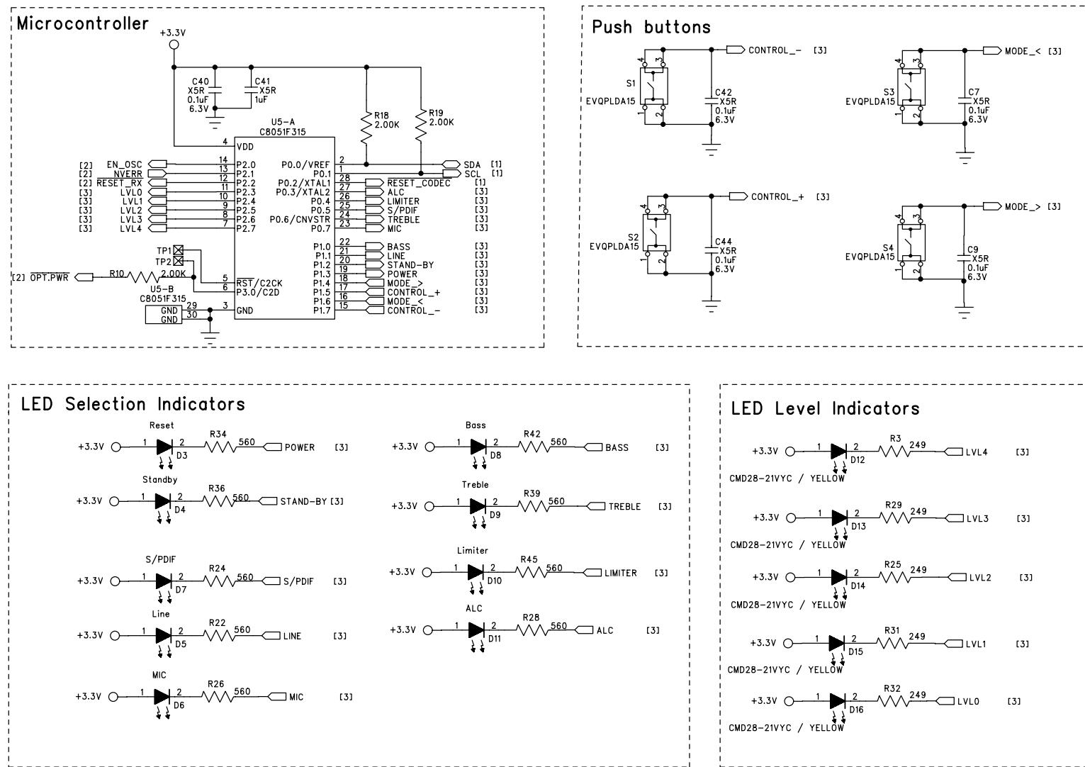
**Figure 4. Microcontroller, Pushbuttons and LED Indicators (Schematic Sheet 3)**
