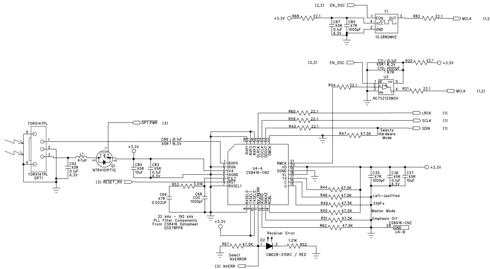
Figure 3. S/PDIF Input (Schematic Sheet 2)
