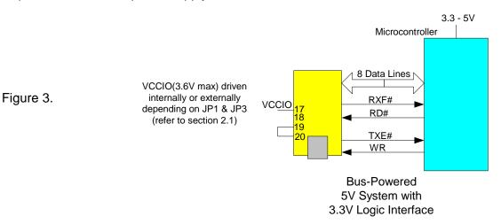
Figure 3 shows how to configure the DLP-2232H to interface with a microcontroller via the parallel 245 FIFO interface mode. In this example, the target electronics can operate at from 3.3 - 5 volts since the DLP-2232H interface I/O pins are 5 volt tolerant.
