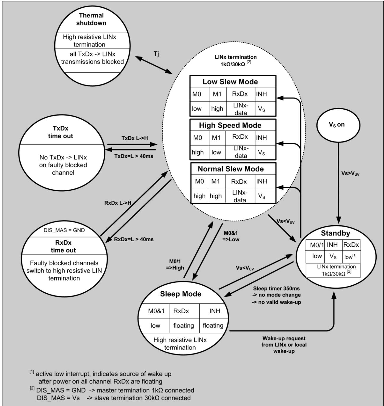
Figure 5: State Diagram of the MLX80004/2
