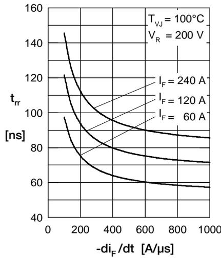
Fig. 5 Typ. recovery time  $t_{rr}$  versus  $-di_F/dt$
