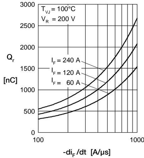
Fig. 2 Typ. reverse recov. charge  $Q_r$  versus  $-di_F/dt$
