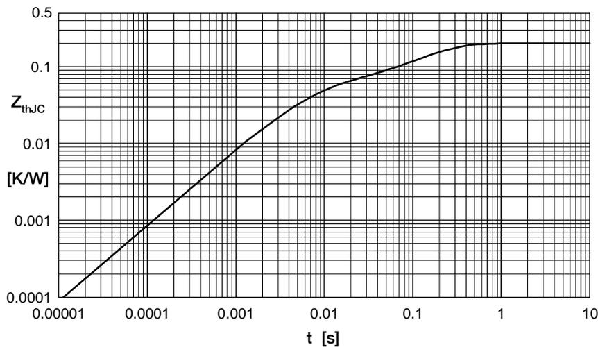
Fig. 7 Transient thermal resistance junction to case
