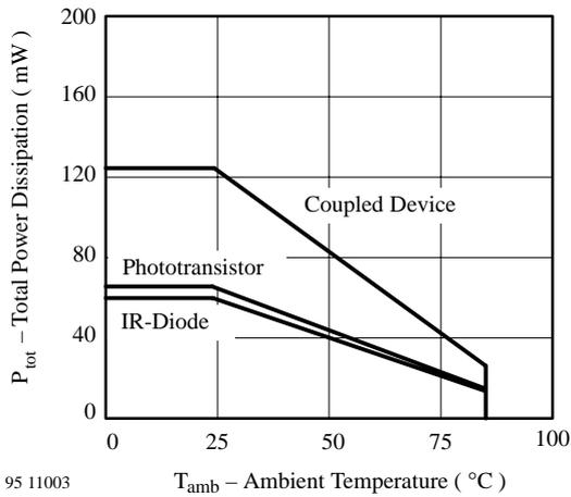
Figure 4. Total Power Dissipation vs. Ambient Temperature
