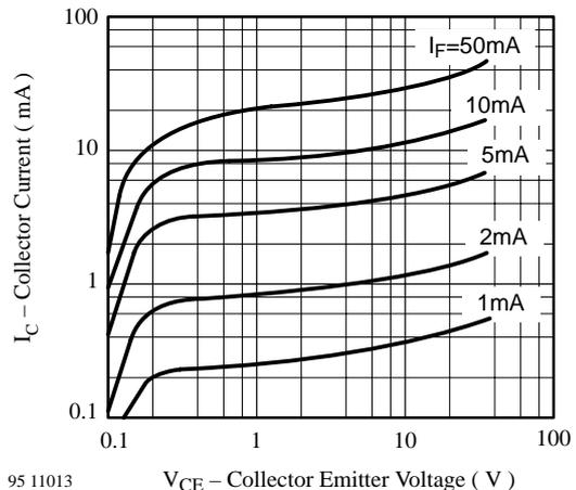
Figure 9. Collector Current vs. Collector Emitter Voltage
