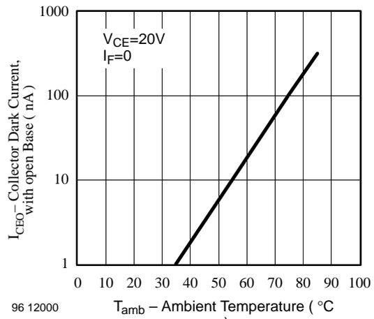
Figure 7. Collector Dark Current vs. Ambient Temperature
