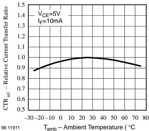
Figure 6. Relative Current Transfer Ratio vs. Ambient Temperature
