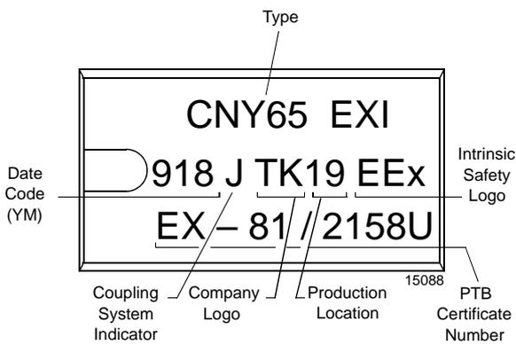
Figure 14. Marking example
