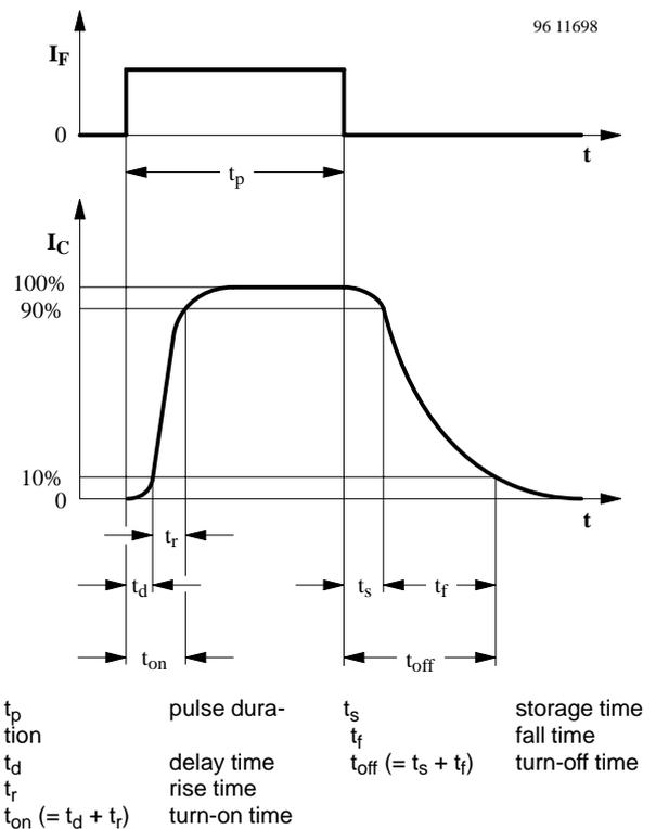
Figure 3. Switching times
