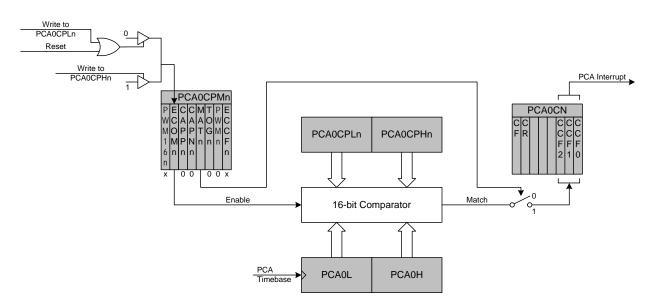
Figure 33.5. PCA Software Timer Mode Diagram
