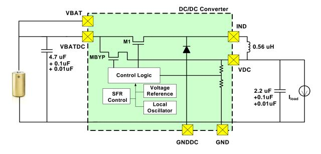
Figure 20.1. Step Down DC-DC Buck Converter Block Diagram
