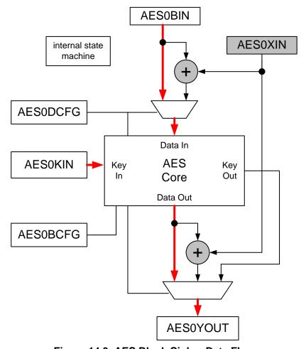
Figure 14.3. AES Block Cipher Data Flow
