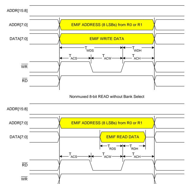
Figure 10.5. Non-multiplexed 8-bit MOVX without Bank Select Timing
