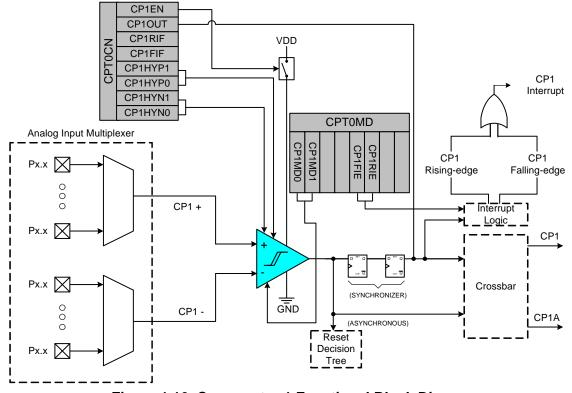
Figure 1.16. Comparator 1 Functional Block Diagram
