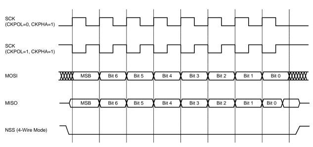
Figure 30.7. Slave Mode Data/Clock Timing (CKPHA = 1)
