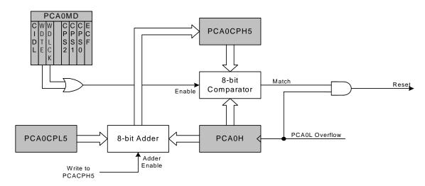
Figure 33.11. PCA Module 5 with Watchdog Timer Enabled
