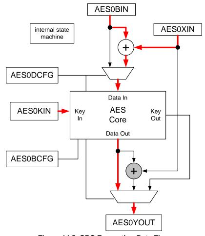
Figure 14.5. CBC Encryption Data Flow
