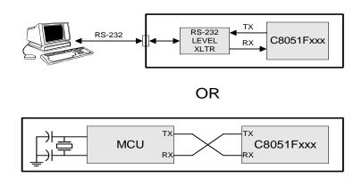
Figure 29.3. UART Interconnect Diagram
