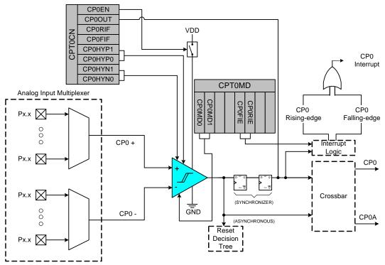
Figure 1.15. Comparator 0 Functional Block Diagram
