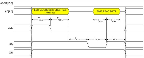
Figure 10.8. Multiplexed 8-bit MOVX without Bank Select Timing
