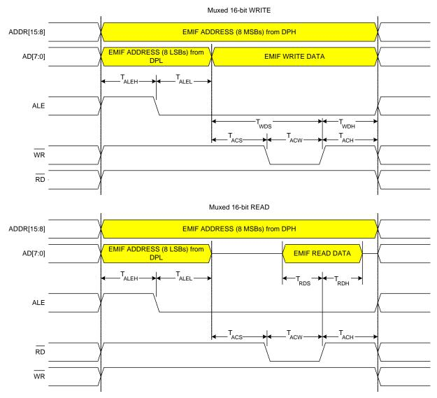
Figure 10.7. Multiplexed 16-bit MOVX Timing
