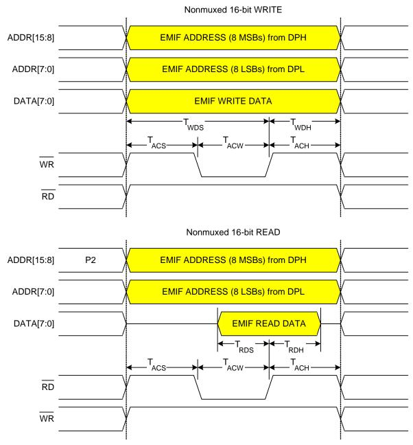
Figure 10.4. Non-multiplexed 16-bit MOVX Timing
