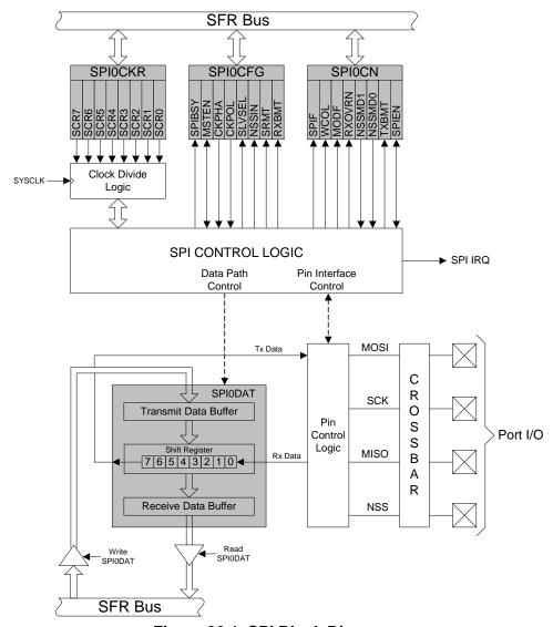
Figure 30.1. SPI Block Diagram
