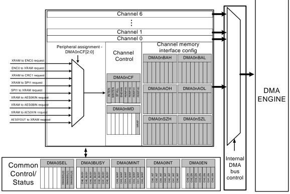
Figure 11.1. DMA0 Block Diagram
