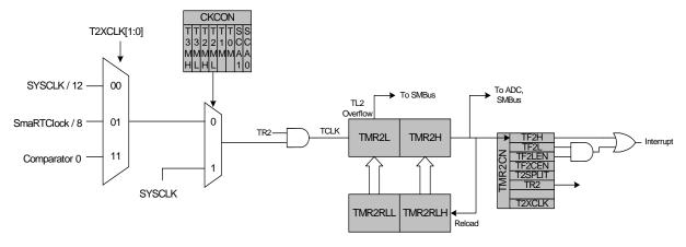
Figure 32.4. Timer 2 16-Bit Mode Block Diagram
