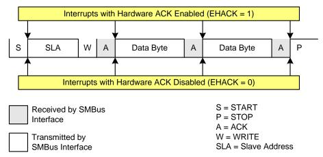
Figure 28.5. Typical Master Write Sequence
