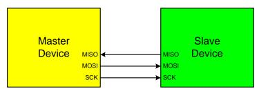
Figure 31.3. 3-Wire Single Master and 3-Wire Single Slave Mode Connection Diagram
