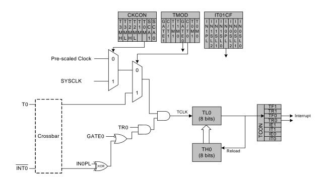
Figure 32.2. T0 Mode 2 Block Diagram
