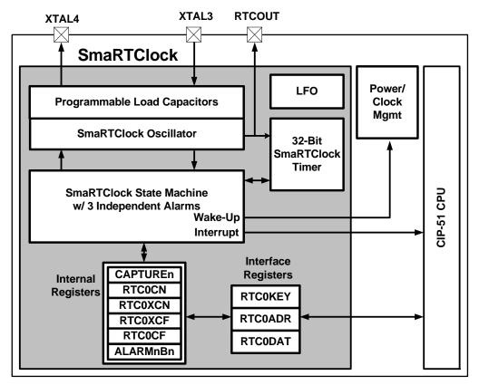
Figure 24.1. SmaRTClock Block Diagram
