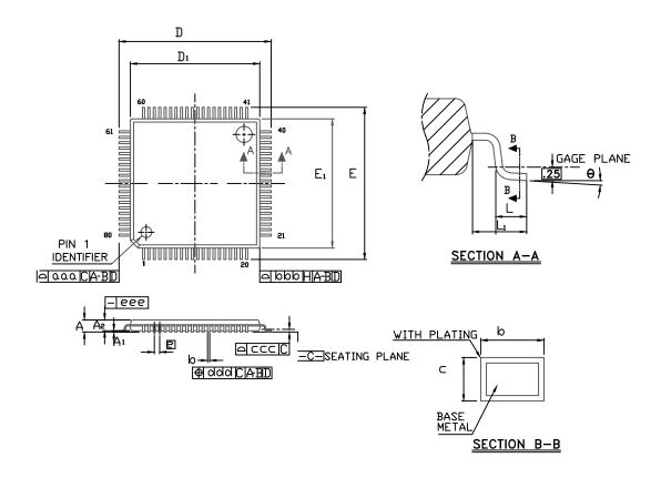
Figure 3.9. TQFP-80 Package Drawing
