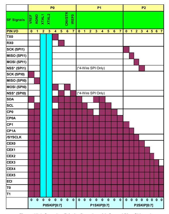
Figure 27.4. Crossbar Priority Decoder with Crystal Pins Skipped
