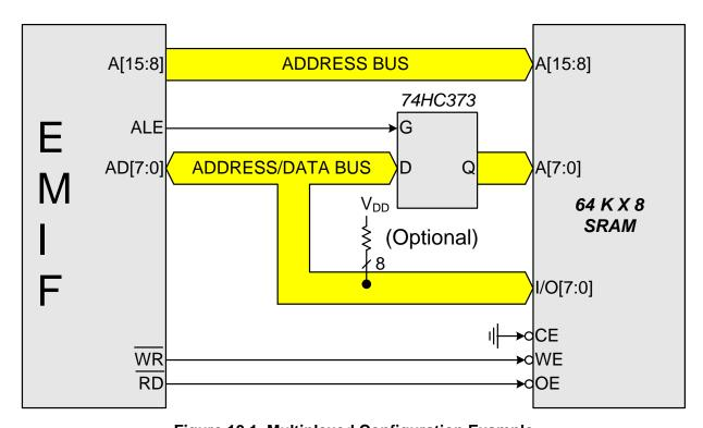
Figure 10.1. Multiplexed Configuration Example
