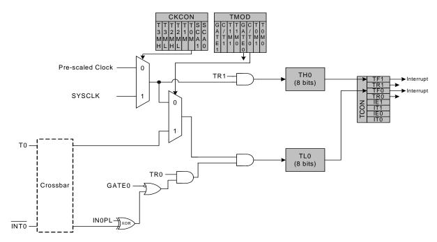
Figure 32.3. T0 Mode 3 Block Diagram
