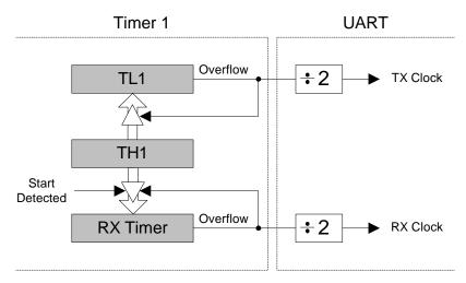
Figure 29.2. UARTO Baud Rate Logic
