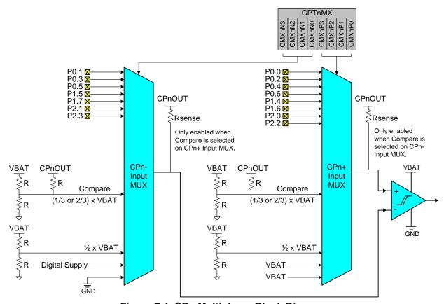
Figure 7.4. CPn Multiplexer Block Diagram
