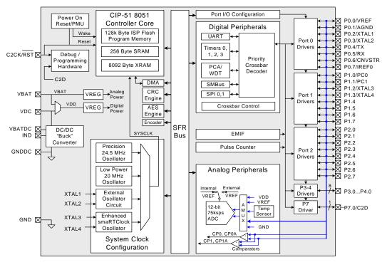
Figure 1.4. C8051F963 Block Diagram
