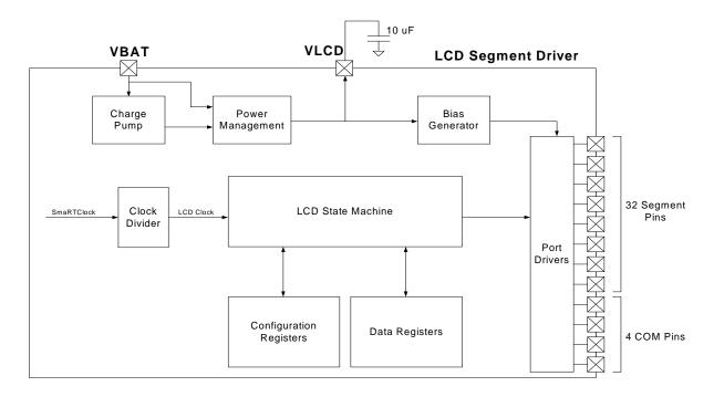
Figure 26.1. LCD Segment Driver Block Diagram
