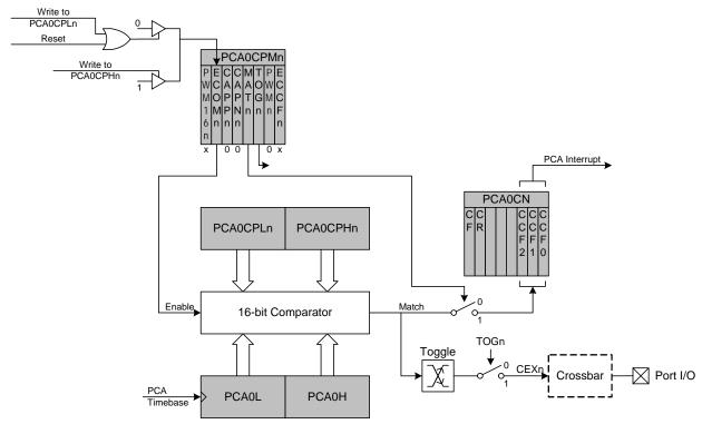
Figure 33.6. PCA High-Speed Output Mode Diagram
