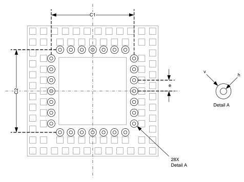
Figure 3.6. Recomended Inner Via Placement
