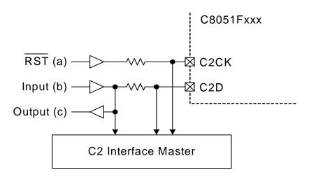
Figure 34.1. Typical C2 Pin Sharing
