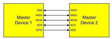
Figure 31.2. Multiple-Master Mode Connection Diagram
