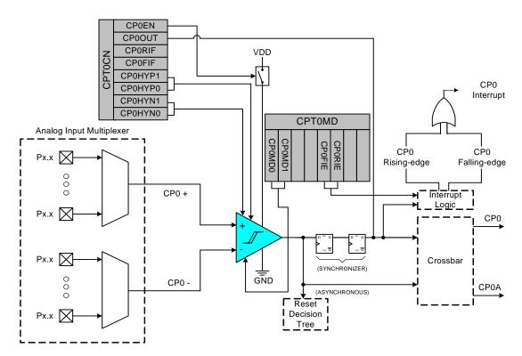
Figure 7.1. Comparator 0 Functional Block Diagram
