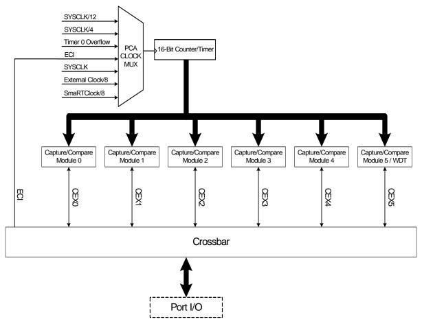
Figure 33.1. PCA Block Diagram
