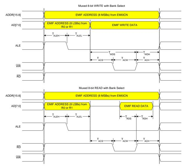
Figure 10.9. Multiplexed 8-bit MOVX with Bank Select Timing
