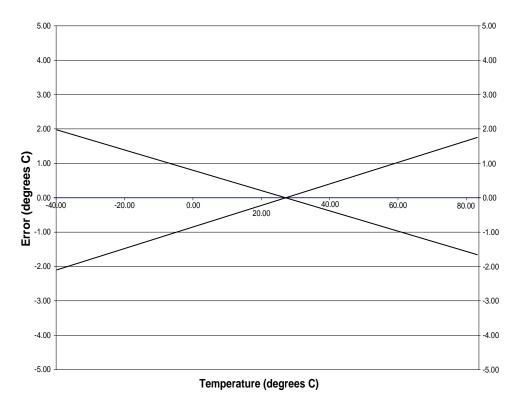
Figure 5.9. Temperature Sensor Error with 1-Point Calibration (V<sub>REF</sub> = 1.68 V)
