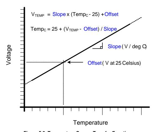
Figure 5.8. Temperature Sensor Transfer Function
