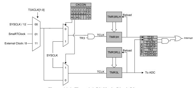
Figure 32.8. Timer 3 8-Bit Mode Block Diagram
