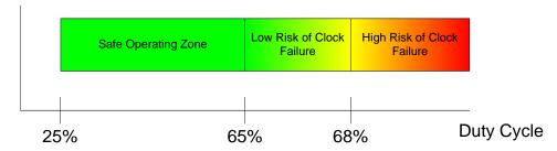
Figure 24.2. Interpreting Oscillation Robustness (Duty Cycle) Test Results
