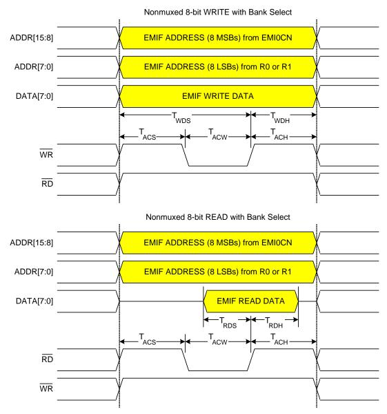
Figure 10.6. Non-multiplexed 8-bit MOVX with Bank Select Timing
