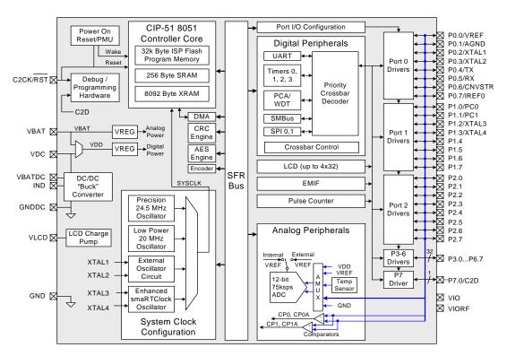
Figure 1.7. C8051F966 Block Diagram
