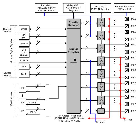
Figure 1.11. Port I/O Functional Block Diagram
