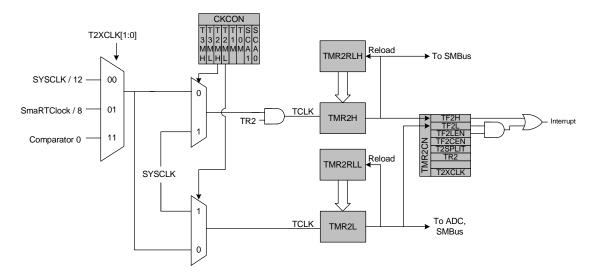
Figure 32.5. Timer 2 8-Bit Mode Block Diagram
