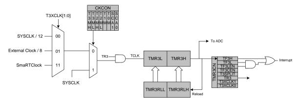
Figure 32.7. Timer 3 16-Bit Mode Block Diagram
