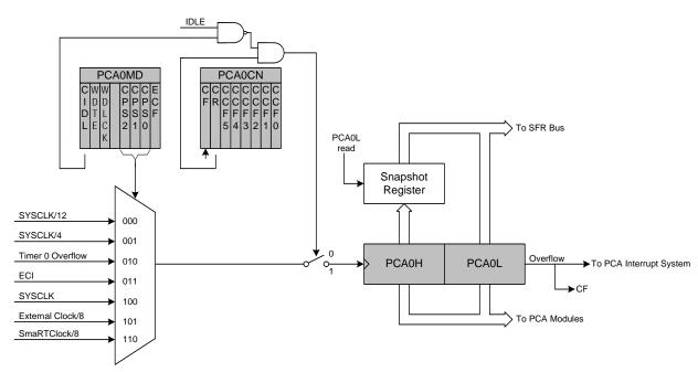
Figure 33.2. PCA Counter/Timer Block Diagram
