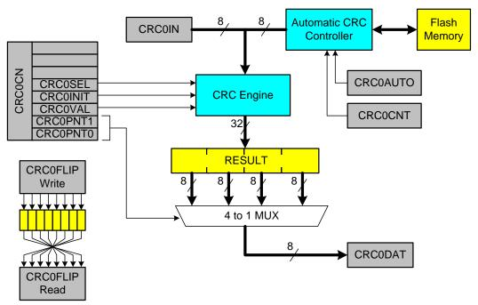
Figure 12.1. CRC0 Block Diagram
