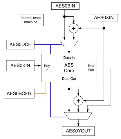
Figure 14.1. AES Peripheral Block Diagram
