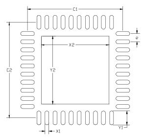
Figure 3.8. QFN-40 Landing Diagram
