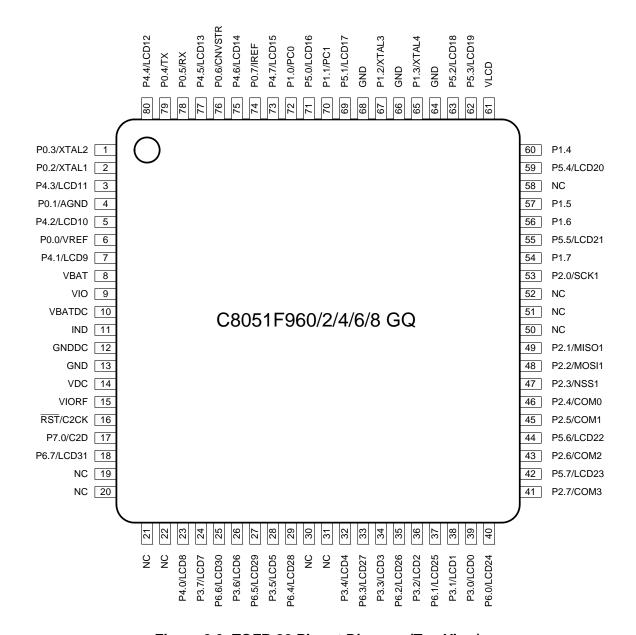
Figure 3.3. TQFP-80 Pinout Diagram (Top View)
