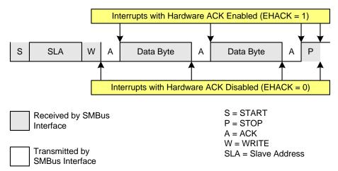
Figure 28.7. Typical Slave Write Sequence
