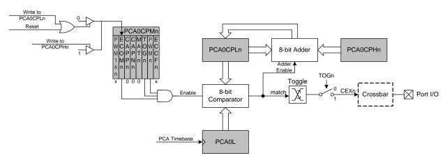
Figure 33.7. PCA Frequency Output Mode
