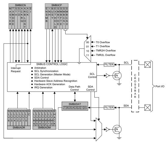
Figure 28.1. SMBus Block Diagram
