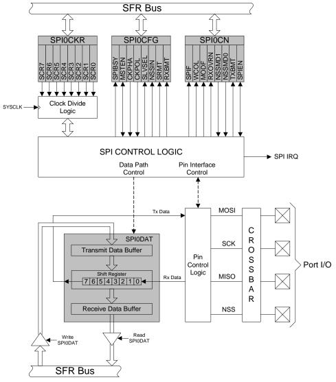
Figure 31.1. SPI Block Diagram
