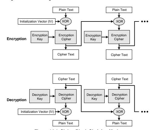
Figure 14.4. Cipher Block Chaining Mode
