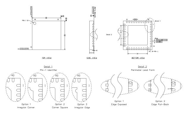
Figure 3.7. Typical QFN-40 Package Drawing
