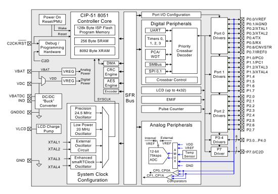
Figure 1.2. C8051F961 Block Diagram
