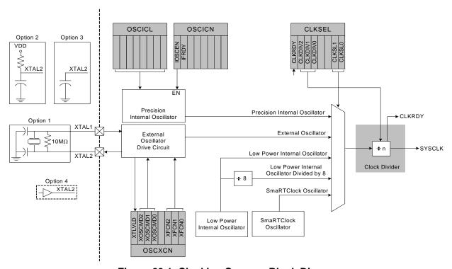
Figure 23.1. Clocking Sources Block Diagram
