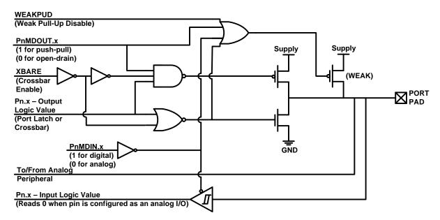
Figure 27.2. Port I/O Cell Block Diagram
