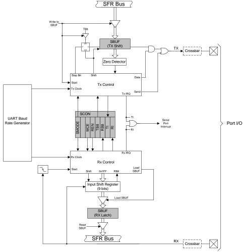
Figure 29.1. UARTO Block Diagram
