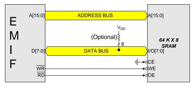
Figure 10.2. Non-multiplexed Configuration Example
