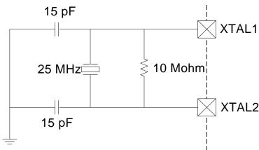
Figure 23.2. 25 MHz External Crystal Example
