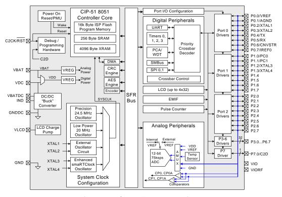
Figure 1.9. C8051F968 Block Diagram
