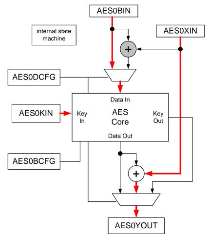
Figure 14.8. Counter Mode Data Flow
