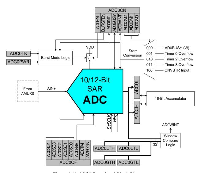
Figure 1.13. ADC0 Functional Block Diagram
