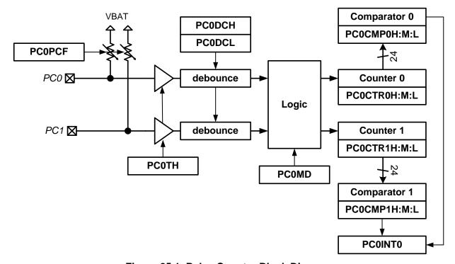
Figure 25.1. Pulse Counter Block Diagram
