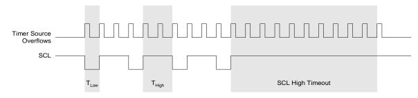
Figure 28.4. Typical SMBus SCL Generation
