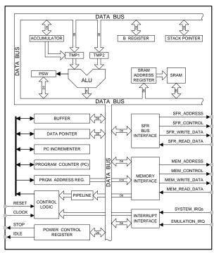
Figure 8.1. CIP-51 Block Diagram
