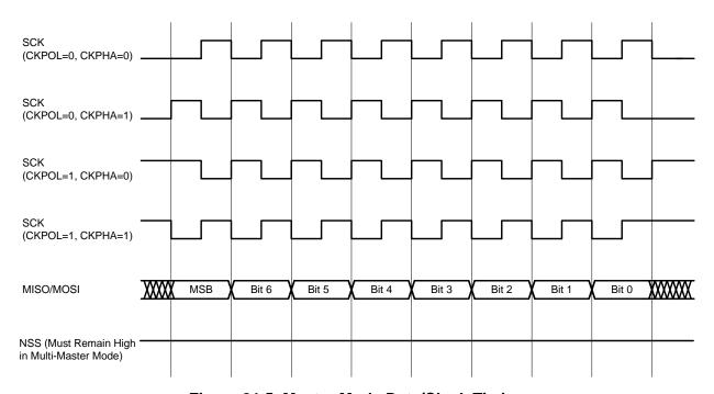
Figure 31.5. Master Mode Data/Clock Timing
