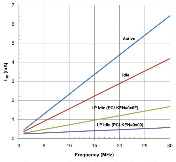
Figure 4.1. Frequency Sensitivity (External CMOS Clock, 25°C)
