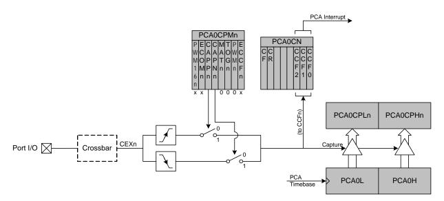
Figure 33.4. PCA Capture Mode Diagram
