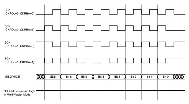
Figure 30.5. Master Mode Data/Clock Timing
