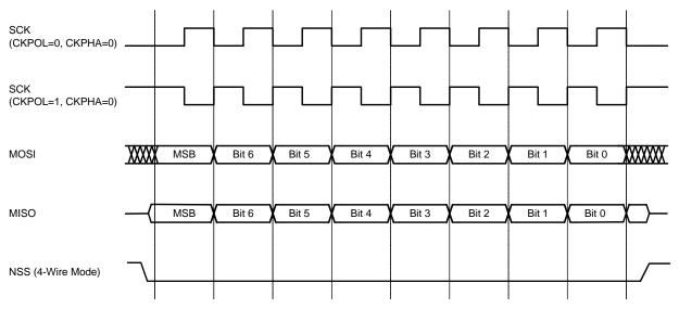
Figure 30.6. Slave Mode Data/Clock Timing (CKPHA = 0)
