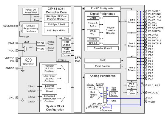
Figure 1.3. C8051F962 Block Diagram
