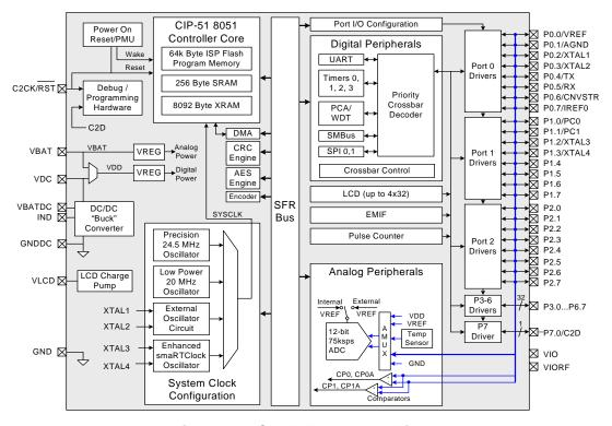
Figure 1.5. C8051F964 Block Diagram
