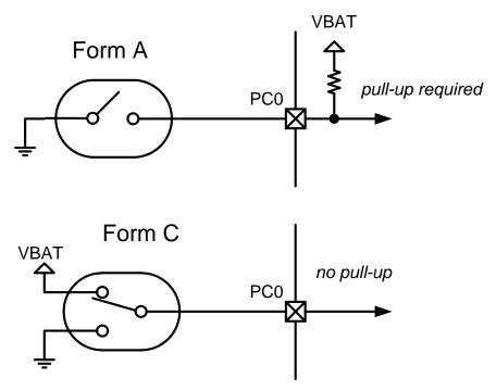
Figure 25.3. Reed Switch Configurations
