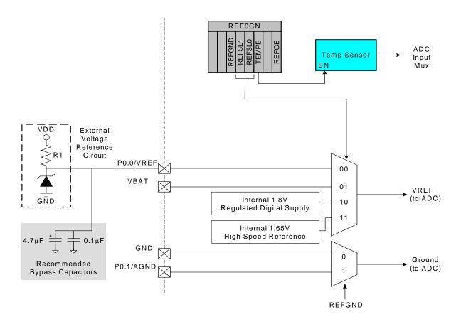
Figure 5.10. Voltage Reference Functional Block Diagram
