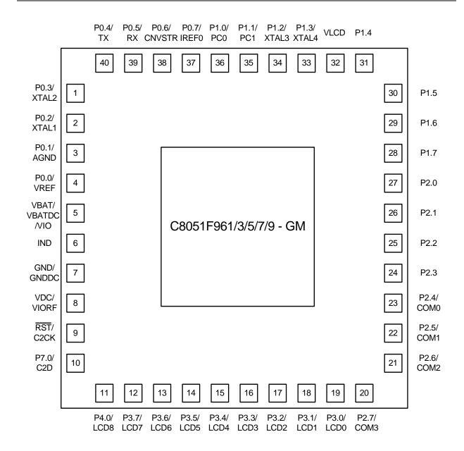
Figure 3.2. QFN-40 Pinout Diagram (Top View)
