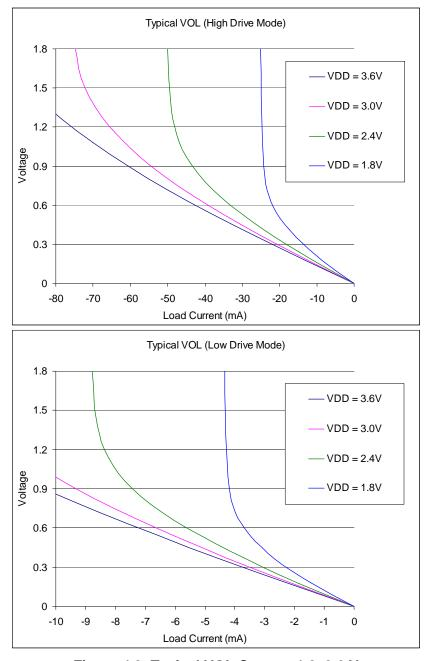
Figure 4.3. Typical VOL Curves, 1.8-3.6 V
