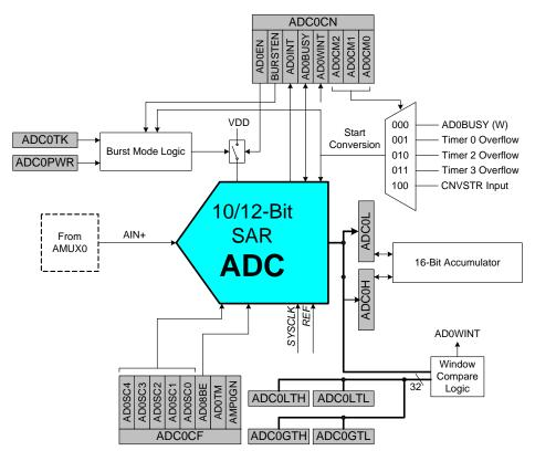
Figure 5.1. ADC0 Functional Block Diagram
