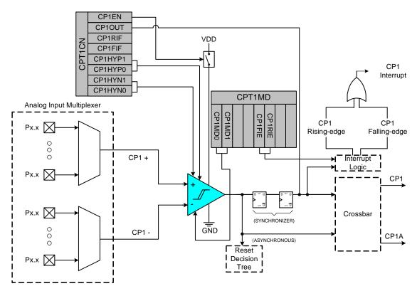
Figure 7.2. Comparator 1 Functional Block Diagram
