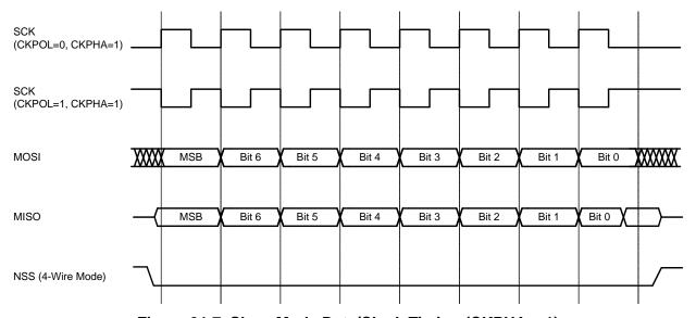
Figure 31.7. Slave Mode Data/Clock Timing (CKPHA = 1)
