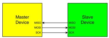
Figure 30.3. 3-Wire Single Master and 3-Wire Single Slave Mode Connection Diagram
