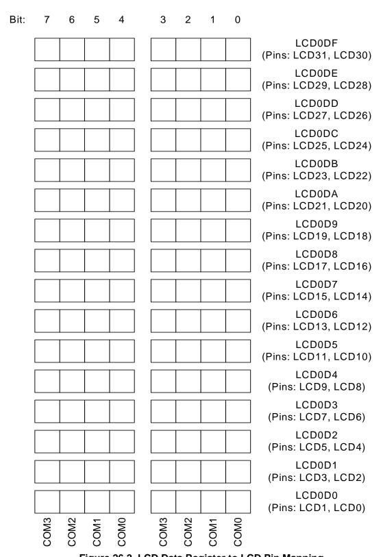
Figure 26.2. LCD Data Register to LCD Pin Mapping
