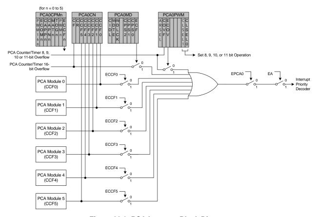
Figure 33.3. PCA Interrupt Block Diagram
