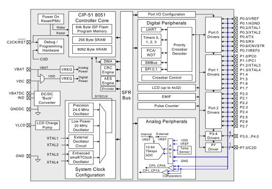
Figure 1.6. C8051F965 Block Diagram
