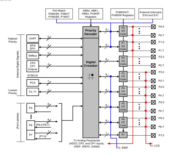
Figure 27.1. Port I/O Functional Block Diagram
