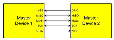
Figure 30.2. Multiple-Master Mode Connection Diagram
