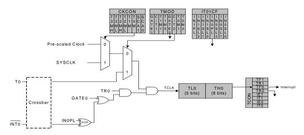
Figure 32.1. T0 Mode 0 Block Diagram
