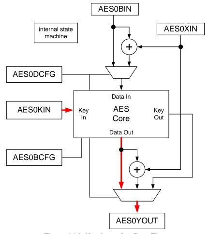
Figure 14.2. Key Inversion Data Flow
