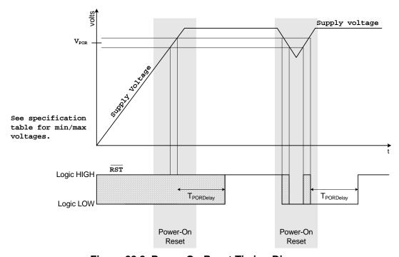
Figure 22.2. Power-On Reset Timing Diagram
