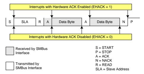
Figure 28.6. Typical Master Read Sequence
