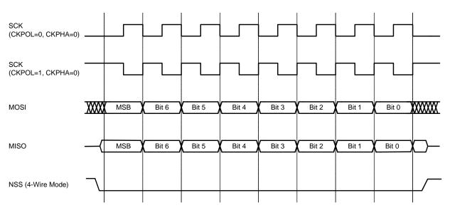
Figure 31.6. Slave Mode Data/Clock Timing (CKPHA = 0)
