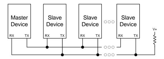
Figure 29.6. UART Multi-Processor Mode Interconnect Diagram
