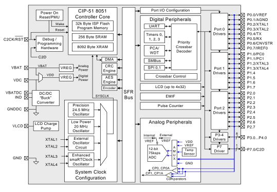
Figure 1.8. C8051F967 Block Diagram
