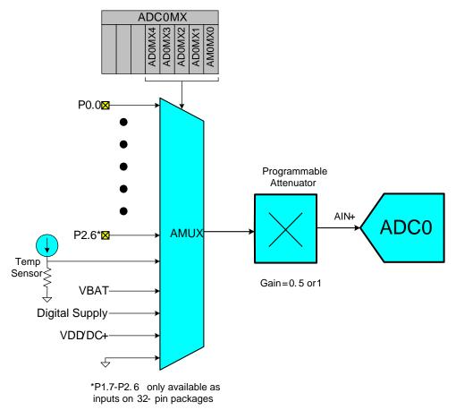
Figure 1.14. ADC0 Multiplexer Block Diagram
