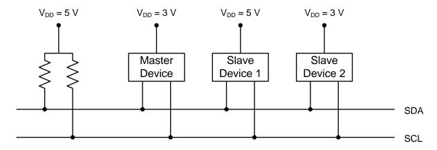
Figure 28.2. Typical SMBus Configuration
