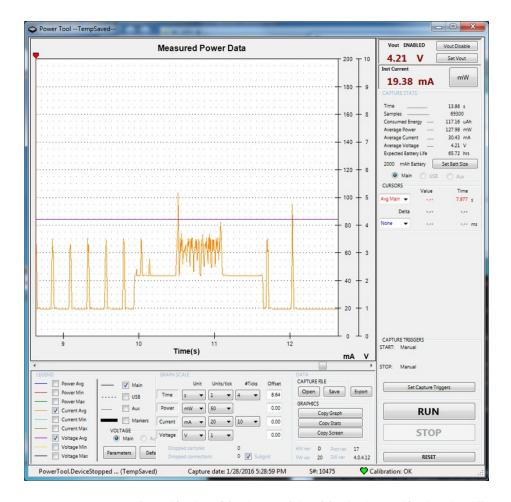
Note that the quiescent current drops from 40mA to 20mA and of that 20mA, about  $^{\sim}12$ mA is the ATmega32u4. Like we said, the best way to really reduce power for long-term usage is to completely turn off the module with KEY
