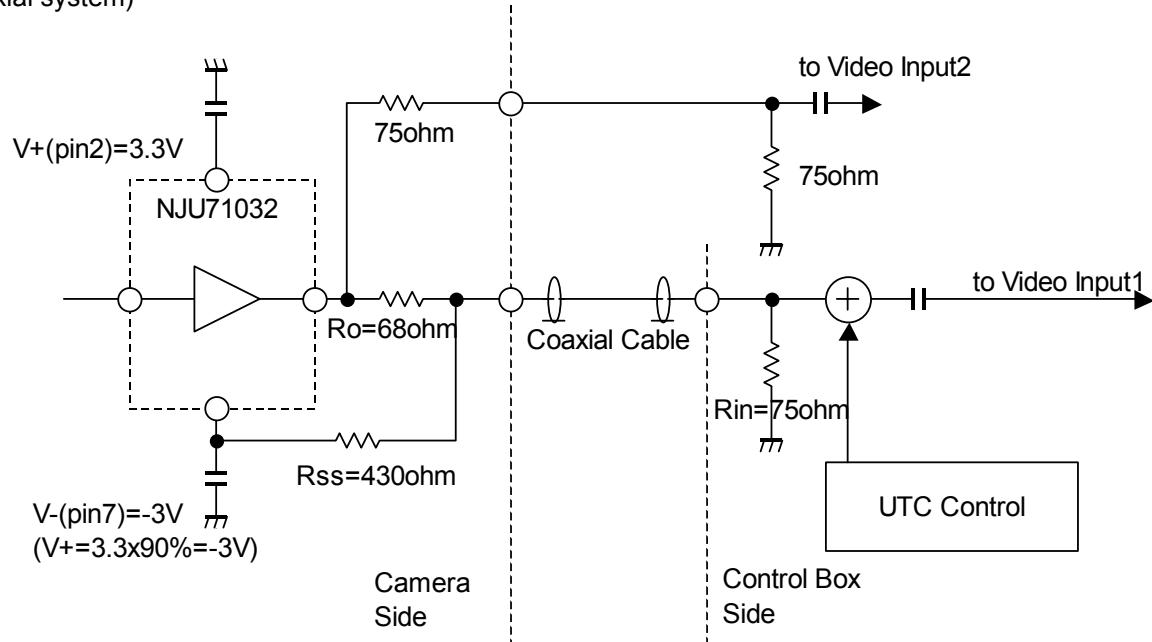
Figure 3: Recommended 2-system drive circuit
