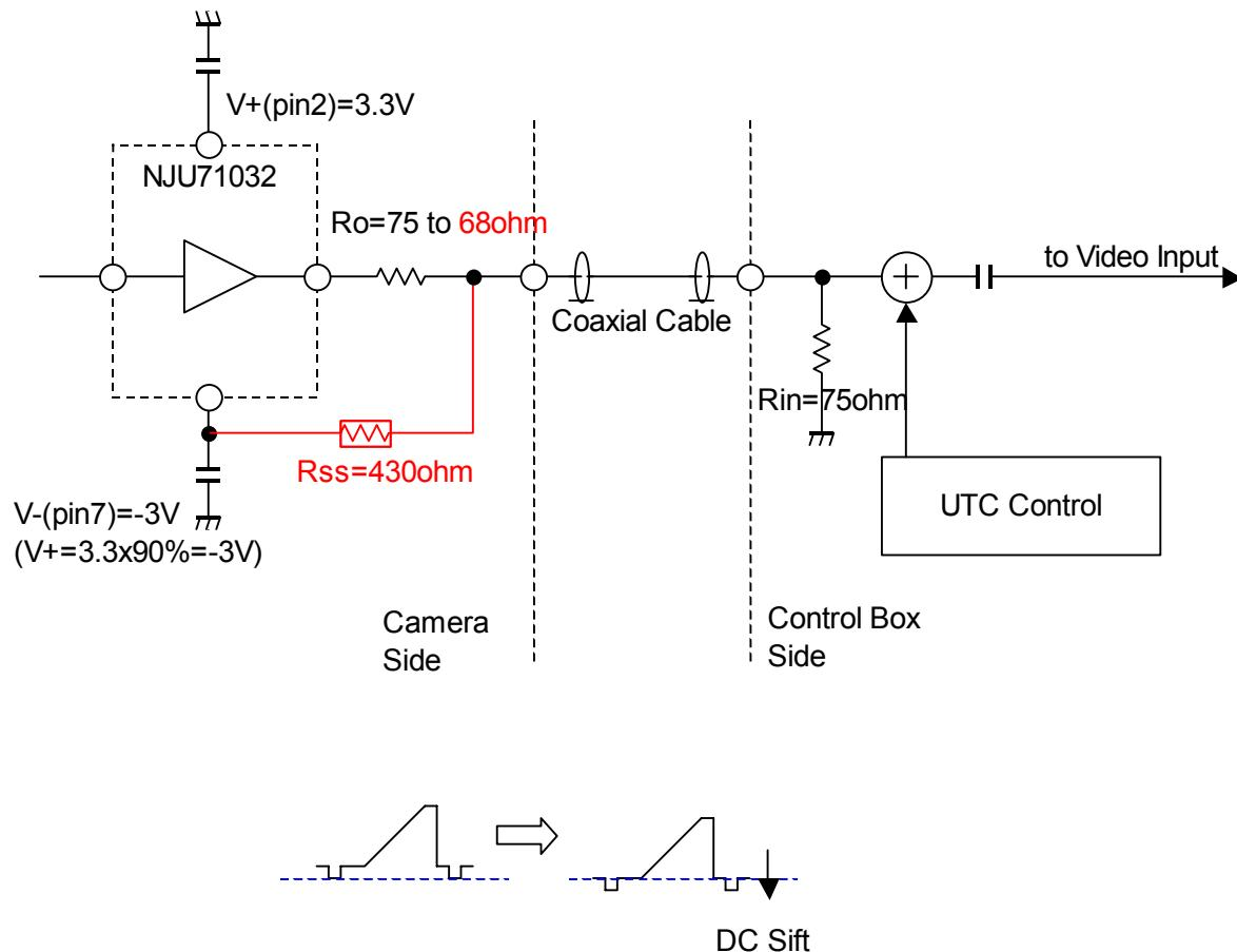
Figure1: How to shift the output DC signal
