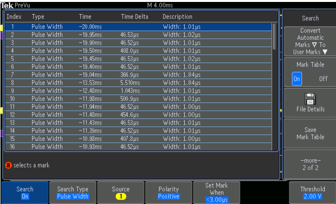
Search step 3: The Search Mark table provides a tabular view of each of the events found by the automated search. Each event is shown with a time stamp making timing measurements between events easy.
