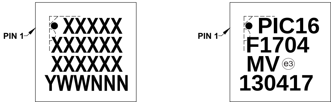
16-Lead QFN (4x4x0.9 mm)
