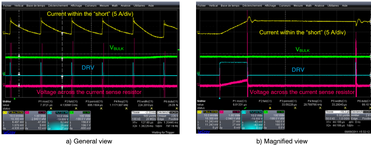
Figure 17. Shorting the Bypass Diode and the NTC
