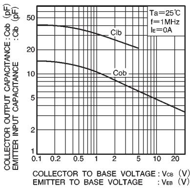
Fig.7 Input/output capacitance vs. voltage
