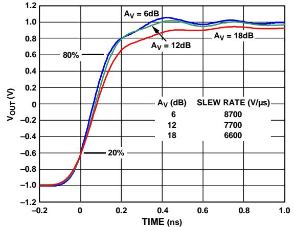
Figure 2. Rise Time,  $V_{OUT} = 2 \text{ V p-p}$ ,  $T_A = 25^\circ\text{C}$ ,
