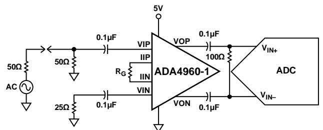
Figure 41. Single-Ended Input Configuration, AC-Coupled to the ADC
