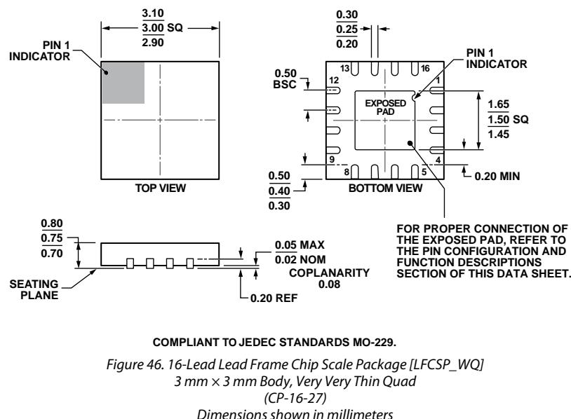
Figure 46. 16-Lead Lead Frame Chip Scale Package [LFCSP\_WQ]
