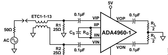
Figure 35. ADA4960-1 with Bandwidth Extension
