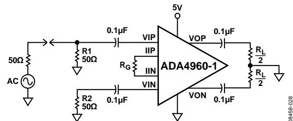
Figure 32. Single-Ended-Input-to-Differential-Output Configuration
