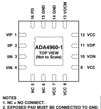
Figure 4. Pin Configuration
