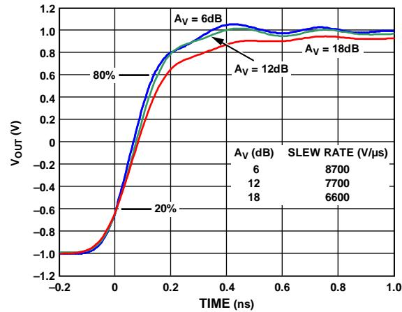
Figure 9. Rise Time, V<sub>OUT</sub> vs. Time, V<sub>OUT</sub> = 2 V p-p
