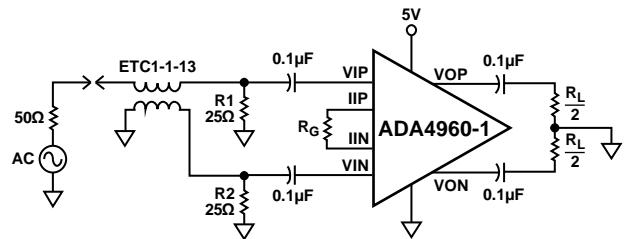
Figure 31. Differential-Input-to-Differential-Output Configuration
