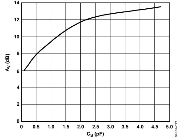
Figure 37. Recommended  $C_S$  Values for Most Gains
