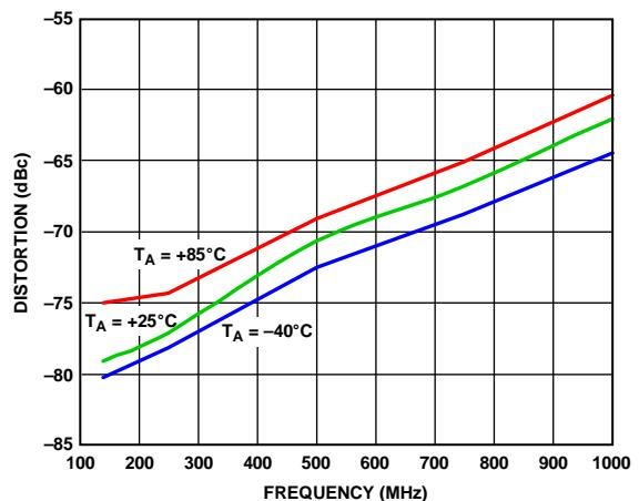
Figure 14. Two Tone IMD3 vs. Frequency at  $T_A = -40^\circ\text{C}$ ,  $T_A = +25^\circ\text{C}$ , and  $T_A = +85^\circ\text{C}$ ,  $A_V = 6\text{ dB}$ ,  $V_{OUT} = 0.45\text{ Vp-p/Tone}$ , 2 MHz Spacing
