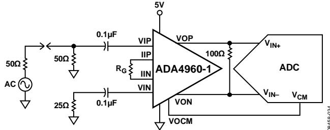
Figure 39. Single-Ended Input Configuration Directly Driving the ADC
