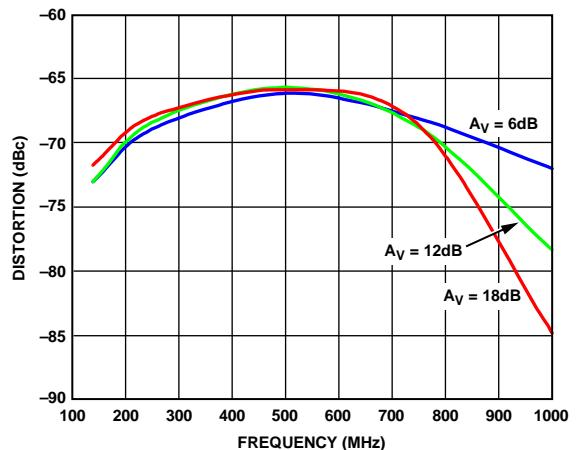
Figure 16. HD3 vs. Frequency at  $A_V = 6\text{ dB}$ ,  $A_V = 12\text{ dB}$ , and  $A_V = 18\text{ dB}$ ,  $V_{OUT} = 0.9\text{ Vp-p}$
