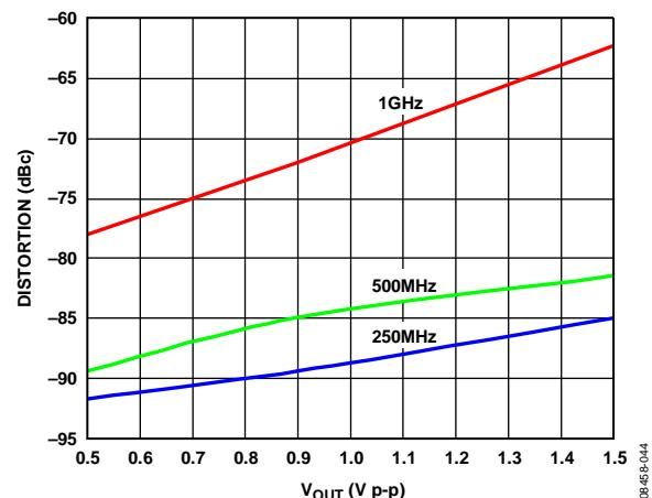
Figure 25. HD2 vs.  $V_{OUT}$  @ 250 MHz, 500 MHz, and 1 GHz,
