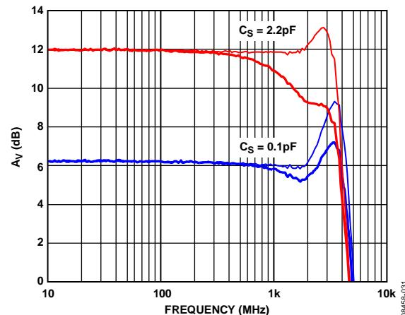
Figure 36. Bandwidth Extension for 6 dB and 12 dB Gains
