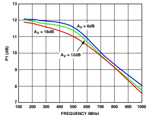
Figure 10. P1dB vs. Frequency at A<sub>V</sub> = 6 dB, A<sub>V</sub> = 12 dB, and A<sub>V</sub> = 18 dB
