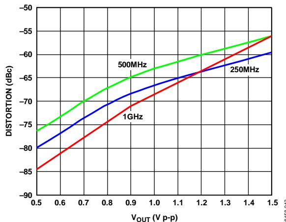
Figure 23. HD3 vs. Output Amplitude @ 250 MHz, 500 MHz, 1 GHz,
