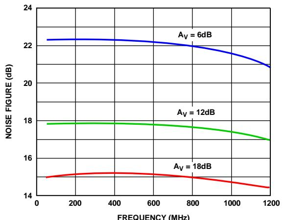
Figure 7. Noise Figure vs. Frequency at A<sub>V</sub> = 6 dB, A<sub>V</sub> = 12 dB, and A<sub>V</sub> = 18 dB
