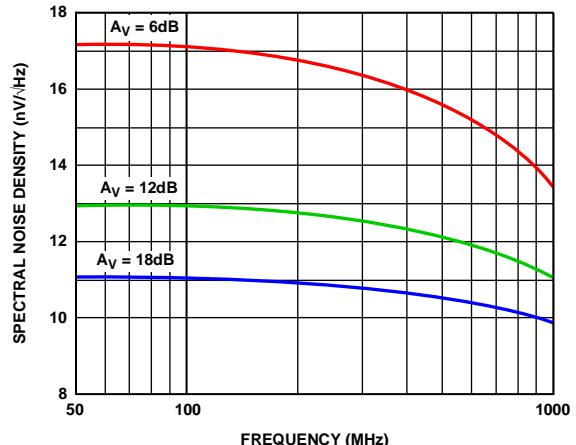
Figure 8. RTO Noise Spectral Density vs. Frequency at
