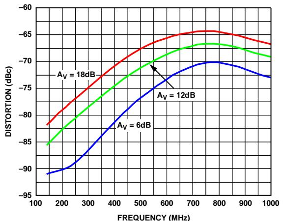
Figure 15. HD2 vs. Frequency at  $A_V = 6\text{ dB}$ ,  $A_V = 12\text{ dB}$ , and  $A_V = 18\text{ dB}$ ,  $V_{OUT} = 0.9\text{ Vp-p}$
