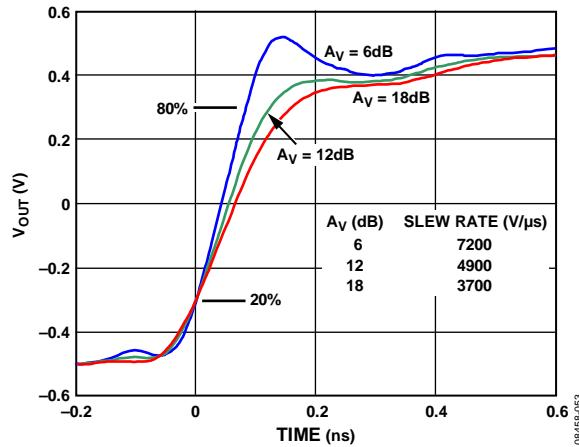
Figure 6. Rise Time, V<sub>OUT</sub> vs. Time, V<sub>OUT</sub> = 1 V p-p
