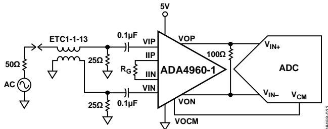
Figure 38. Differential Input Configuration Directly Driving the ADC
