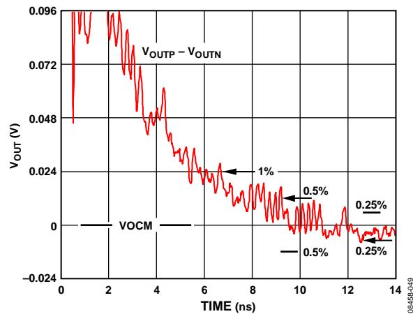
Figure 26. Output Overdrive Recovery,  $V_{OUT}$  vs. Time,
