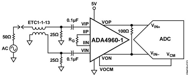
Figure 38. Differential Input Configuration Directly Driving the ADC
