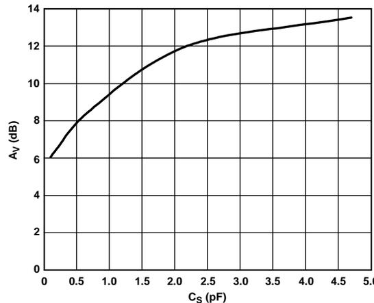
Figure 37. Recommended  $C_S$  Values for Most Gains
