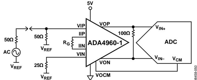
Figure 40. Single-Ended Input Configuration, DC-Coupled Inputs and Outputs
