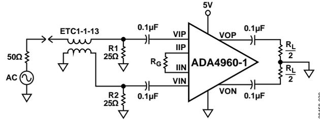
Figure 31. Differential-Input-to-Differential-Output Configuration
