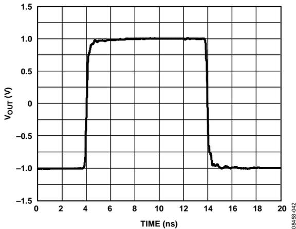
Figure 18. Large Signal Pulse Response,  $A_V = 18\text{ dB}$
