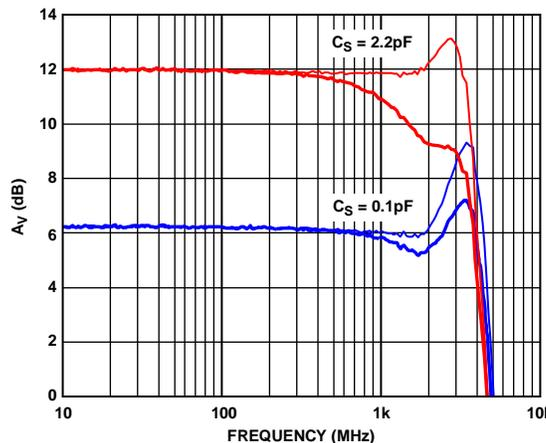
Figure 36. Bandwidth Extension for 6 dB and 12 dB Gains
