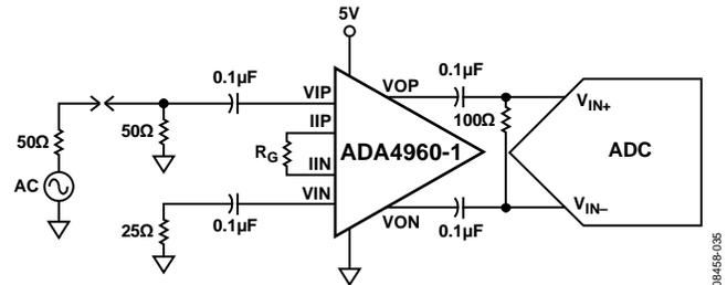
Figure 41. Single-Ended Input Configuration, AC-Coupled to the ADC
