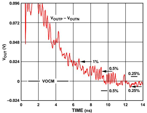
Figure 43. Output Overdrive Recovery
