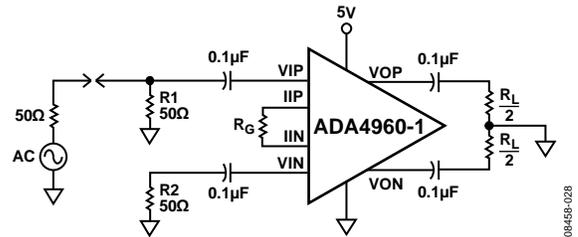
Figure 32. Single-Ended-Input-to-Differential-Output Configuration
