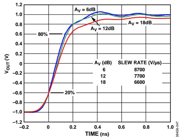
Figure 2. Rise Time,  $V_{OUT} = 2$  V p-p,  $T_A = 25^\circ\text{C}$ ,
