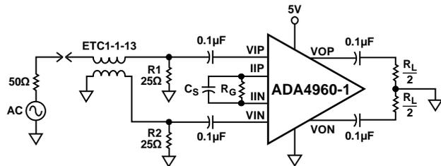
Figure 35. ADA4960-1 with Bandwidth Extension
