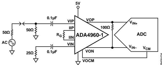
Figure 39. Single-Ended Input Configuration Directly Driving the ADC
