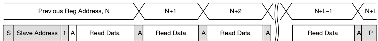
Figure 42. Sequential READ, Start from Current Location
