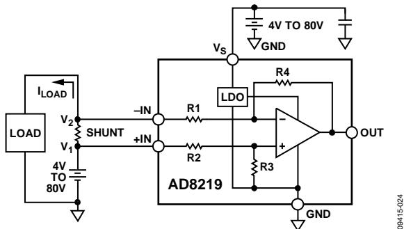
Figure 26. Simplified Schematic
