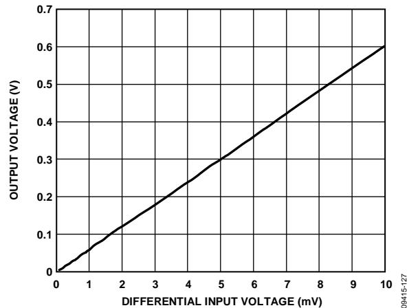
Figure 27. Typical Gain Linearity at Small Differential Inputs
