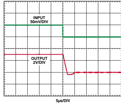
Figure 14. Fall Time (Differential Input = 50 mV)
