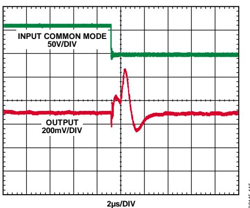
Figure 21. Common-Mode Step Response (Falling)
