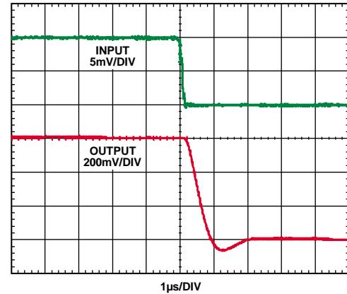
Figure 13. Fall Time (Differential Input = 5 mV)
