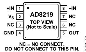
Figure 2. Pin Configuration
