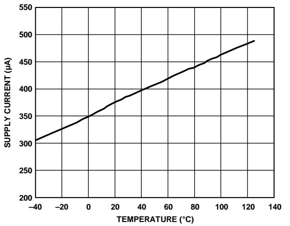
Figure 10. Typical Supply Current Change over Temperature ( $V_S = 5 V$ )
