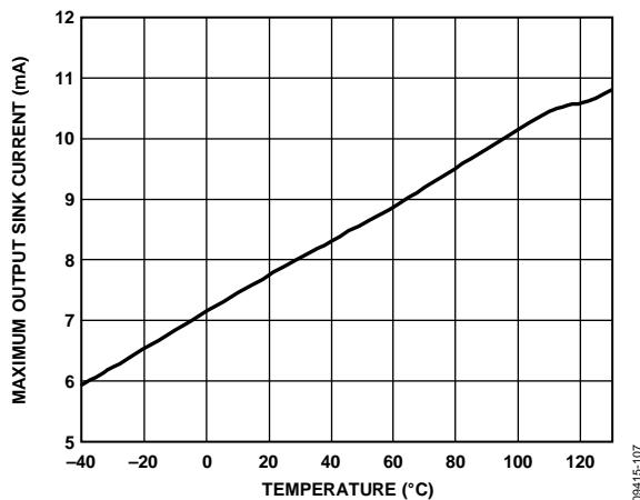
Figure 17. Maximum Output Sink Current vs. Temperature
