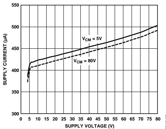
Figure 9. Typical Supply Current vs. Supply Voltage ( $V_S$  Connected to  $+IN$ )
