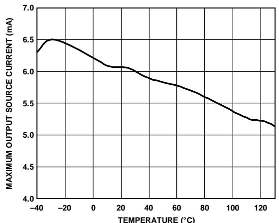
Figure 18. Maximum Output Source Current vs. Temperature
