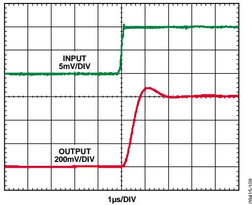
Figure 11. Rise Time (Differential Input = 5 mV)
