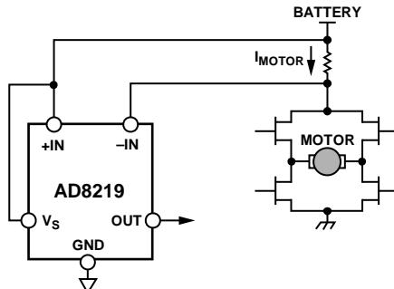
Figure 30. High-Side Current Sensing in Motor Control
