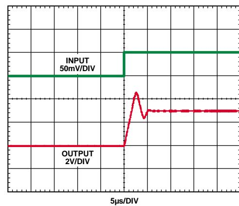
Figure 12. Rise Time (Differential Input = 50 mV)
