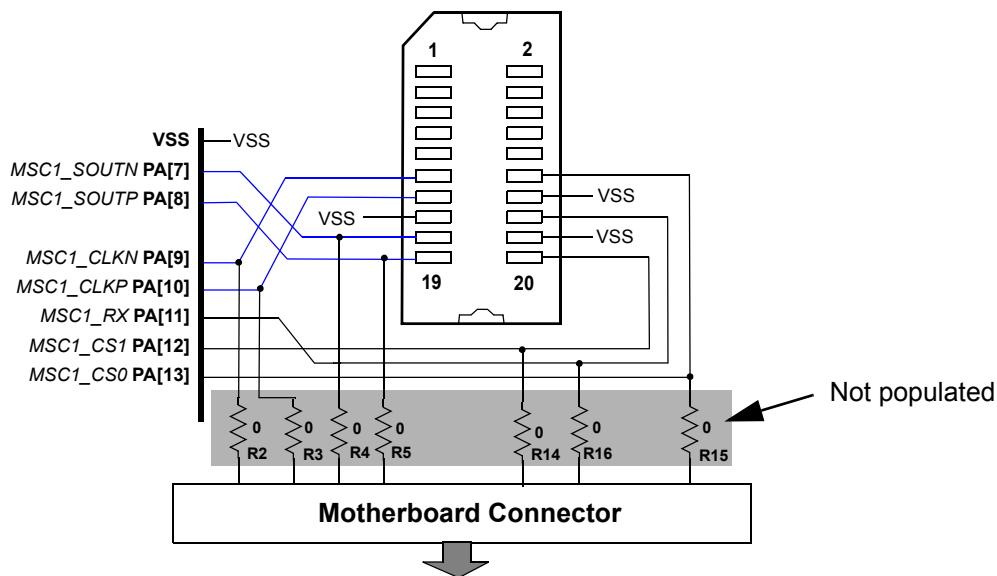
**Figure 2. Samtech ERF8 - MSC1 Connections (20-pin)**
