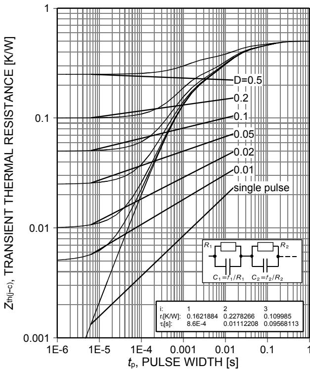
Figure 18. IGBT transient thermal resistance
