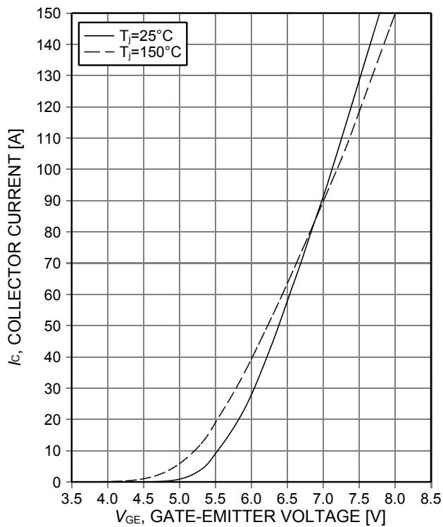
**Figure 6. Typical transfer characteristic**
