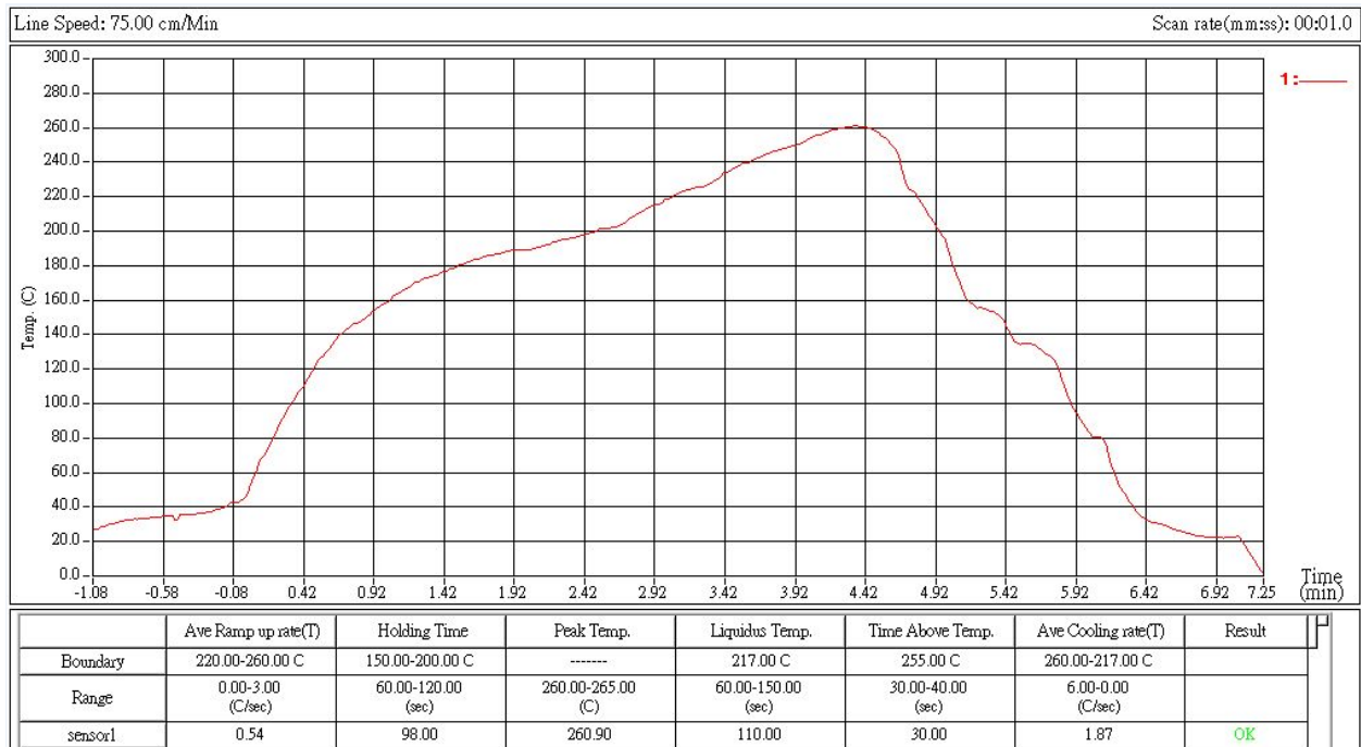
Figure 8.5 Solder Reflow Profile
