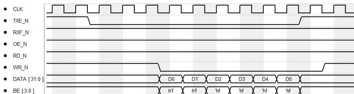
Figure 4.7 245 Synchronous FIFO mode bus master write cycle
