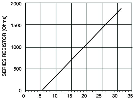
**SERIES LIMIT BIAS RESISTOR VS BIAS VOLTAGE**
