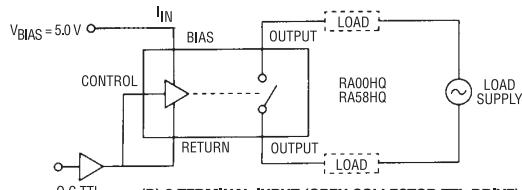
**(B) 2 TERMINAL INPUT (OPEN COLLECTOR TTL DRIVE)**
