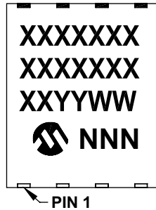
8-Lead DFN-S (6x5x0.9 mm)
