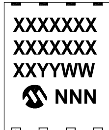
8-Lead DFN-S (6x5x0.9 mm)
