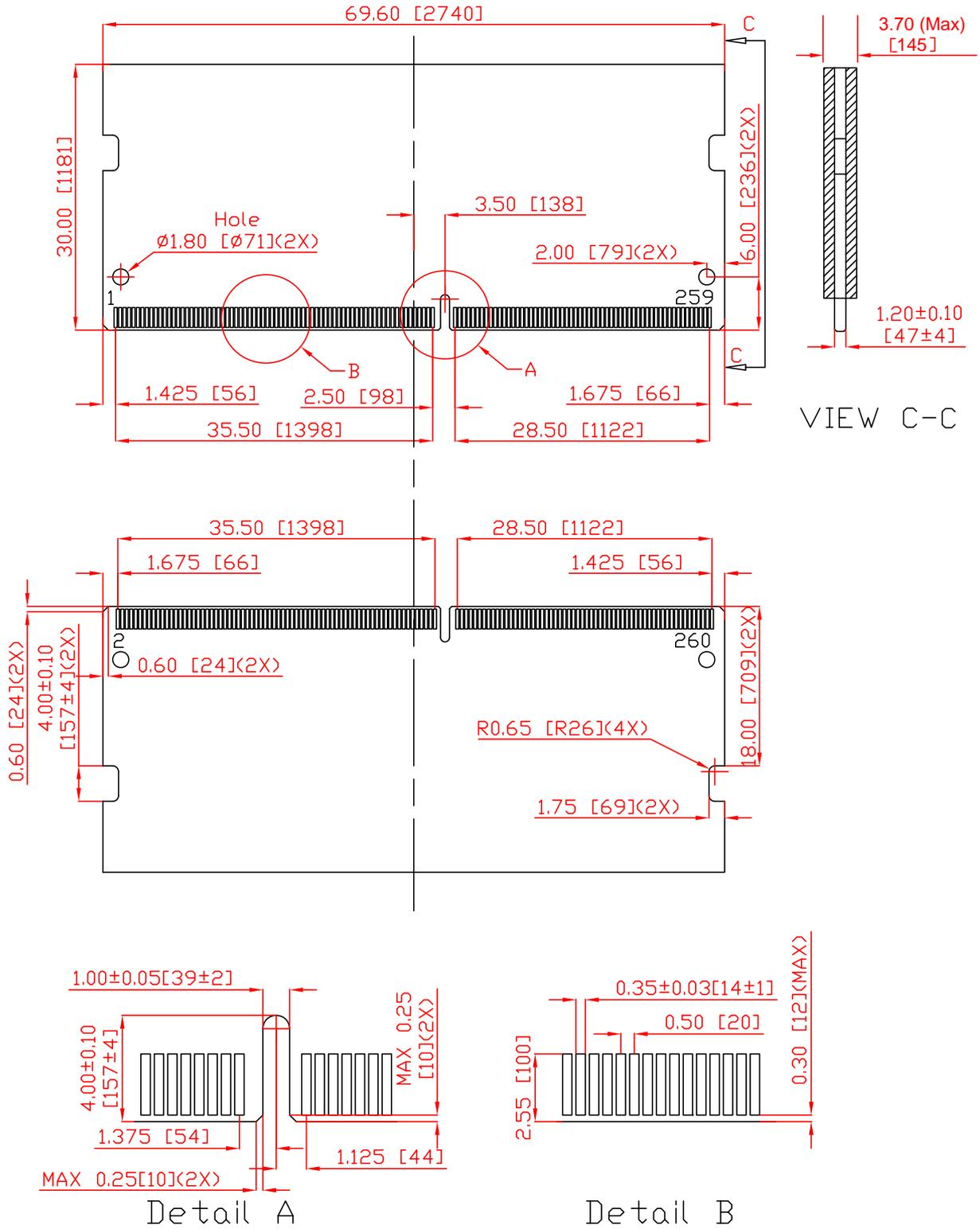
(All dimensions are in millimeters with ±0.15mm tolerance unless specified otherwise.)
