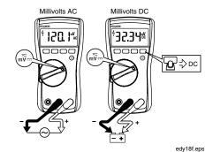
With the function switch in the  $\overline{_{nV}}$ ... position, the Meter measures ac plus dc millivolts. Press \_\_\_\_\_ to switch the Meter to dc millivolts.
