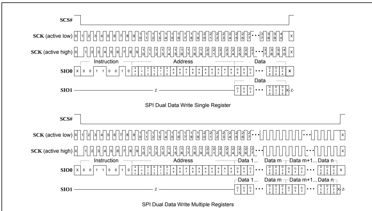
FIGURE 10-13: SPI DUAL DATA WRITE
