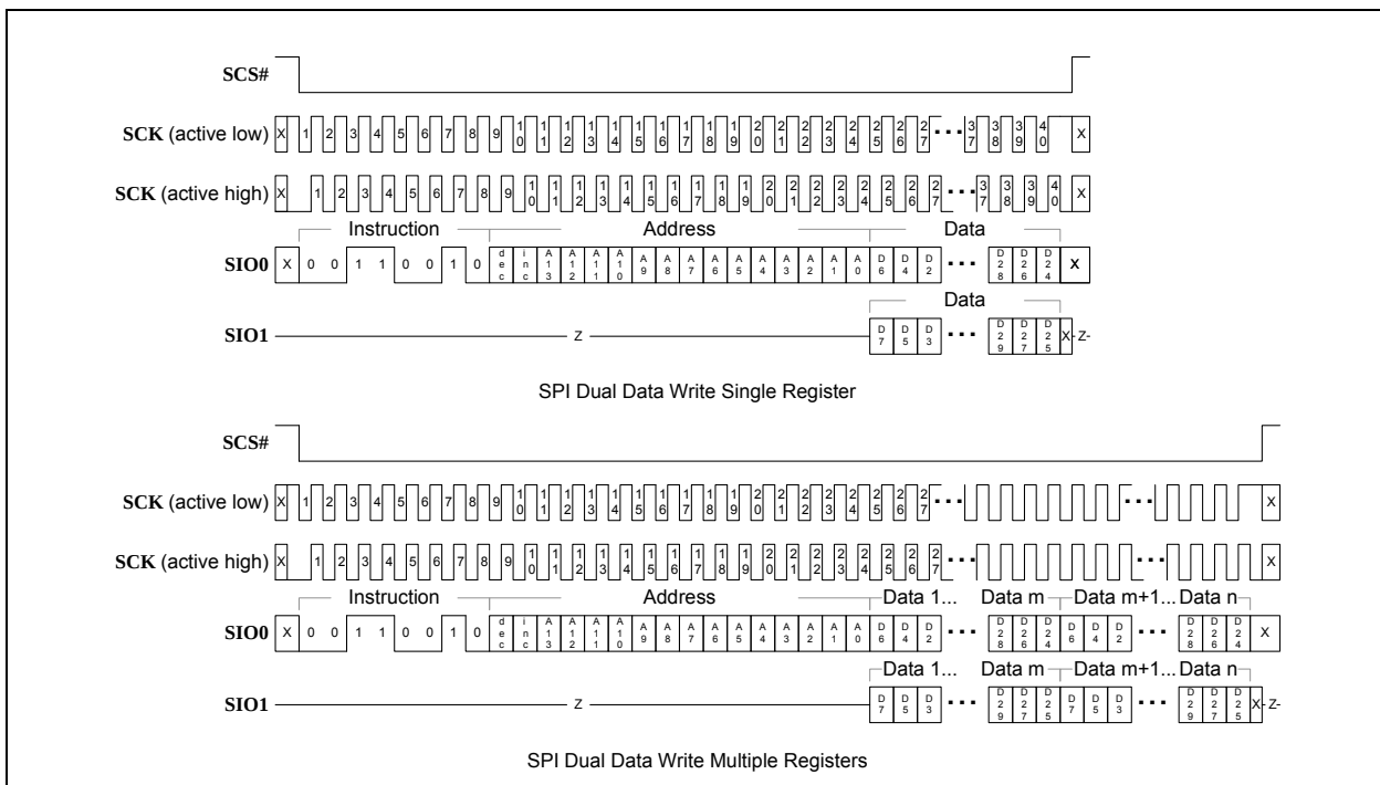
FIGURE 10-13: SPI DUAL DATA WRITE
