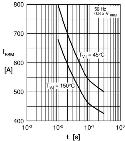
Fig. 2 Surge overload current vs. time per diode
