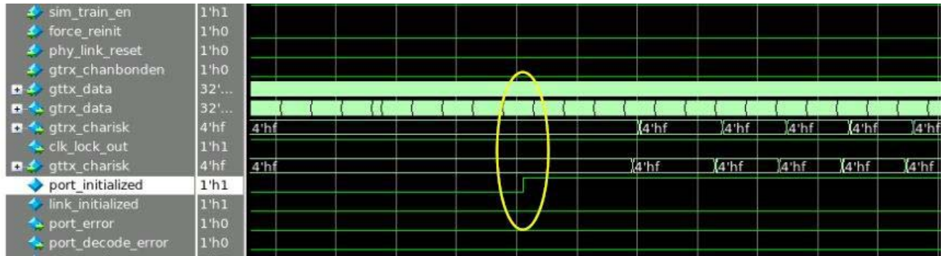
Figure C-3: port_initialized and link_initialized Signals
