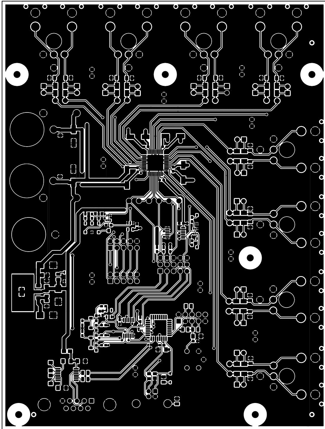
Figure 12. Top Side Copper Layer
