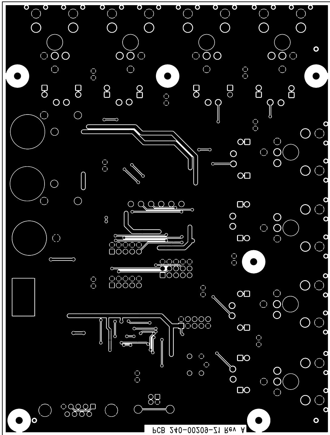
Figure 13. Bottom Side Copper Layer
