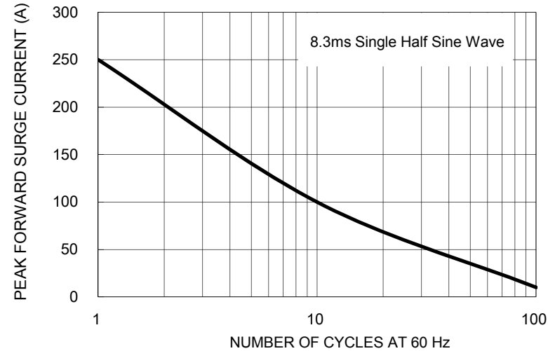
FIG. 9- MAXIMUM NON-REPETITIVE PEAK FORWARD SURGE CURRENT
