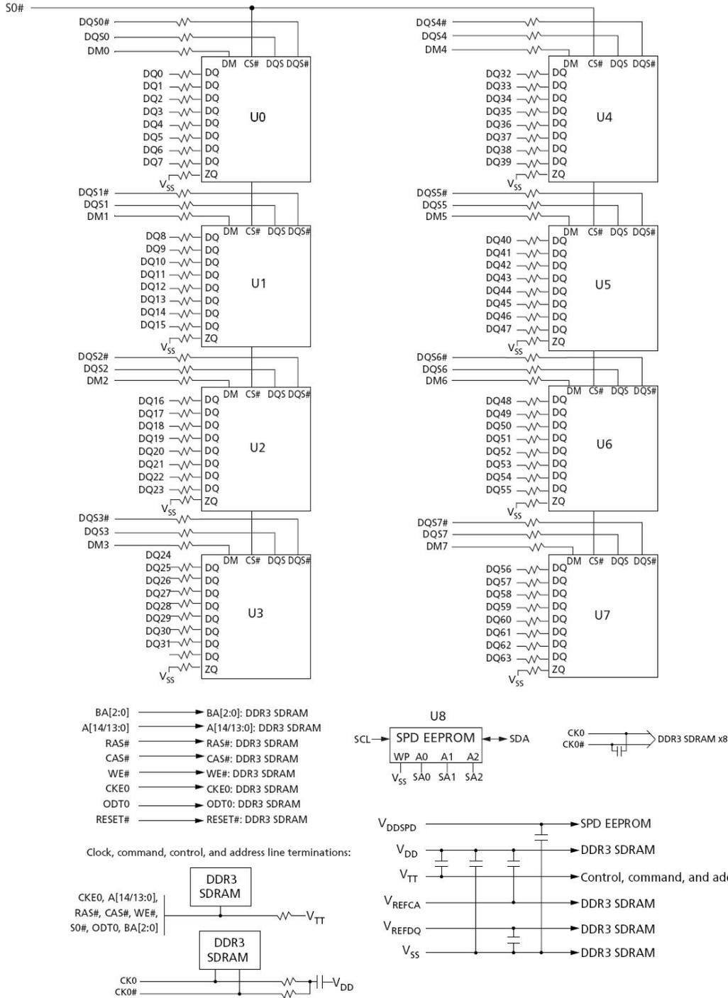
Note: 1. The ZQ ball on each DDR3 component is connected to an external 240Ω ±1% resistor that is tied to ground. It is used for the calibration of the component's ODT and output driver.
