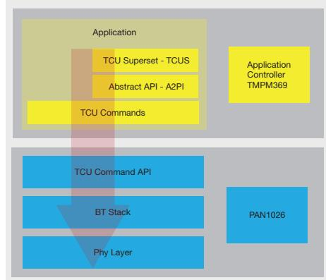
1. This design is intended only for software development and should not be used as hardware reference design. For optimum performance, the module should be on the edge of the application PCB. For layout recommendations and how to place the module refer to the PAN1026 design guide.
