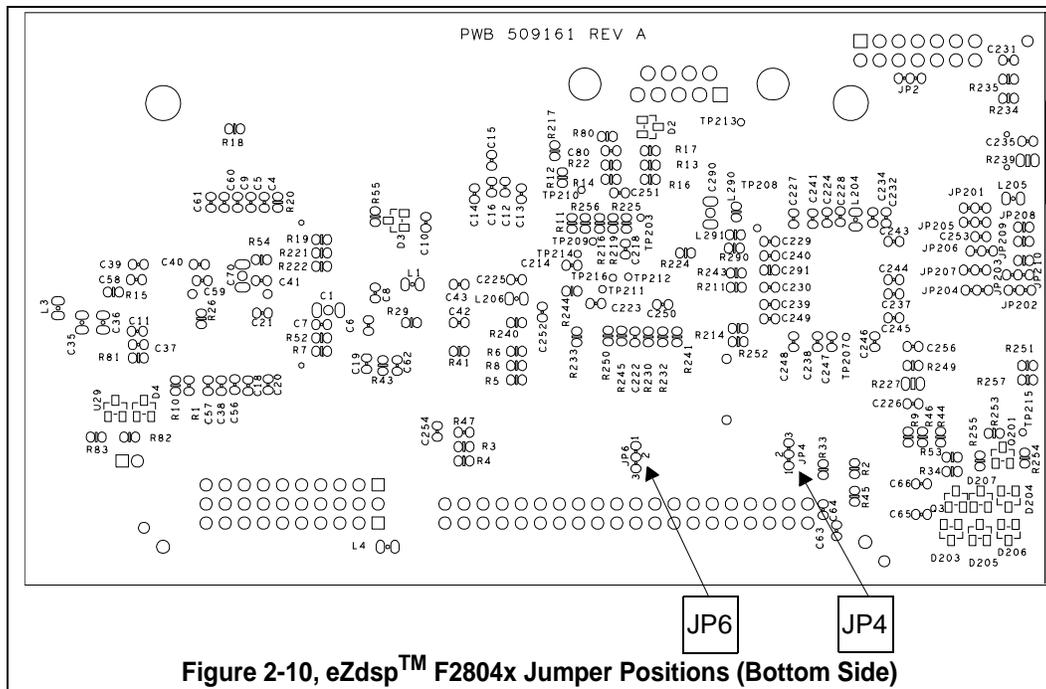
**Figure 2-10, eZdsp™ F2804x Jumper Positions (Bottom Side)**
