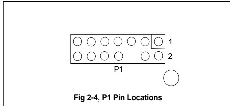
The definition of P1, which has the JTAG signals is shown below.
