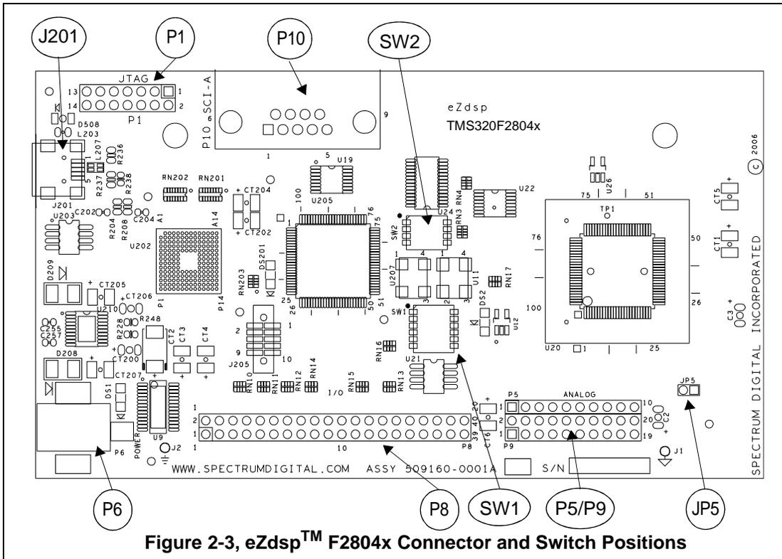
Figure 2-3, eZdsp™ F2804x Connector and Switch Positions
