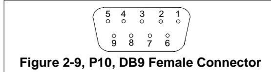
The pin numbers and their corresponding signals are shown in the table below. This corresponds to a standard dual row to DB-9 connector interface used on personal computers.
