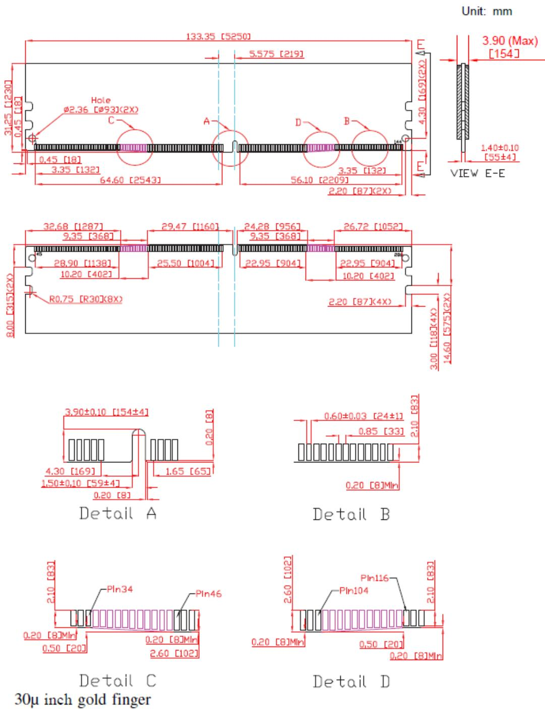
(All dimensions are in millimeters with  $\pm 0.15\text{mm}$  tolerance unless specified otherwise.)
