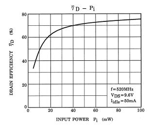
Note 3: These are only typical curves and devices are not necessarily guaranteed at these curves.
